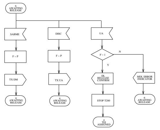
Figure 3.7-5 — Link Layer Point-to-Point: State 6, Awaiting Release (1 of 2)
