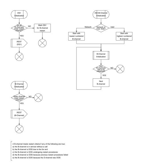
Figure 9.3-10 — National ISDN PRI with BCAS: DS1, DS1/B-channel, and B-channel Initialization Procedures
