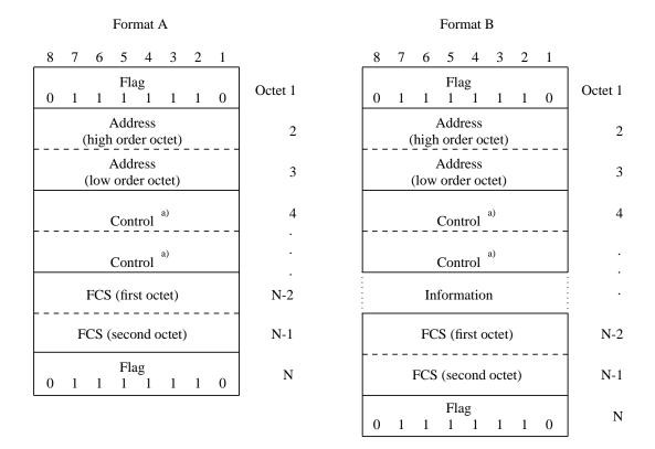
a) Unacknowledged operation Multiple frame operation - one octet
