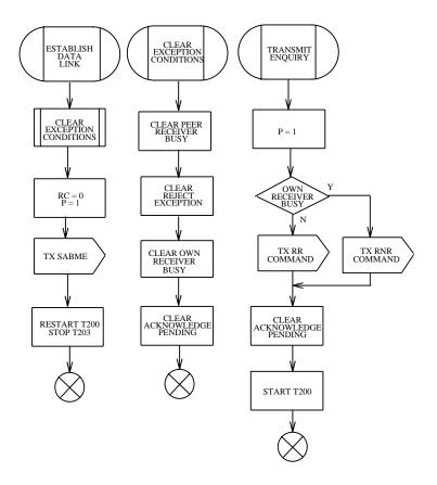
Figure 3.7-9 — Link Layer Point-to-Point: Procedures (2 of 3)
