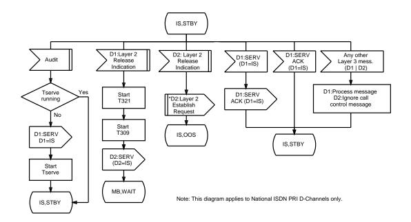
Figure 9.3-26 — National ISDN PRI with D-channel Backup: In Service, Standby (1 of 2)
