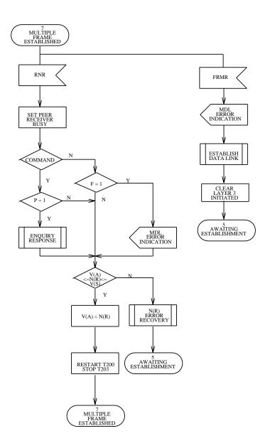
Figure 3.7-6 — Link Layer Point-to-Point: State 7, Multiple Frame Established (5 of 8)
