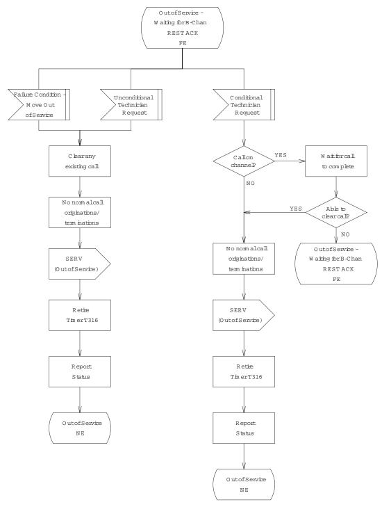
Figure 9.3-24 — National ISDN PRI with BCAS: B-channels, Out of Service FE, Waiting for B-channel REST ACK (3 of 4)
