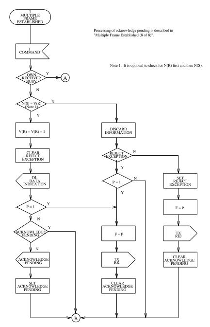
Figure 3.7-6 — Link Layer Point-to-Point: State 7, Multiple Frame Established (6 of 8)
