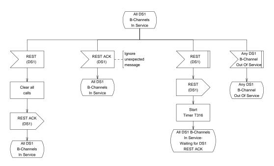
Figure 9.3-14 — National ISDN PRI with BCAS: DS1, All B-channels In Service State (1 of 2)
