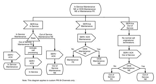
Figure 9.2-4 — Custom ISDN PRI: In Service Maintenance State (1 of 4)
