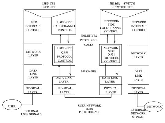
a. Protocol Stack diagram of Elements Between User and Network
