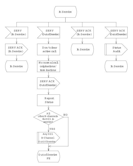
Figure 9.3-19 — National ISDN PRI with BCAS: B-channels, In Service (1 of 3)
