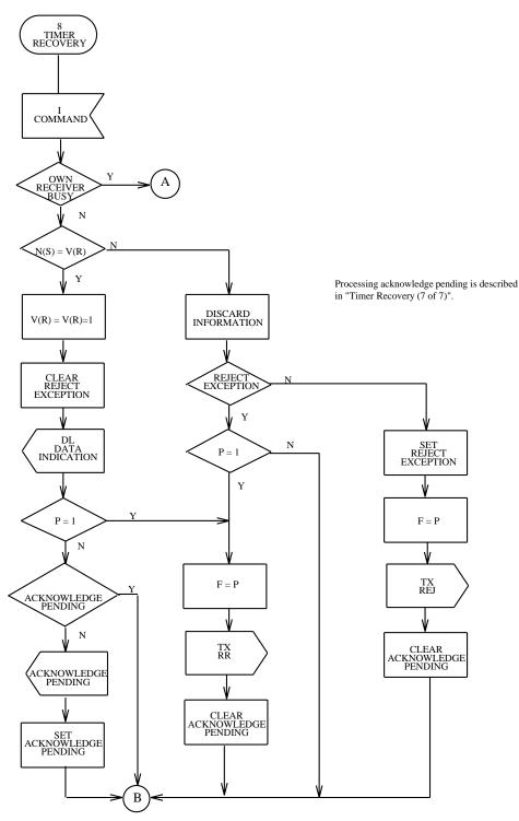
Figure 3.7-7 — Link Layer Point-to-Point: State 8, Timer Recovery (5 of 7)
