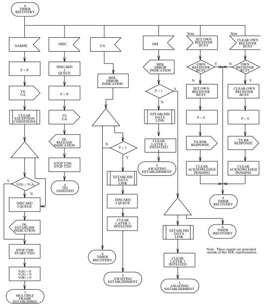
Figure 3.7-7 — Link Layer Point-to-Point: State 8, Timer Recovery (2 of 7)
