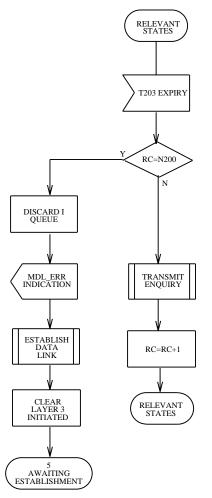
Figure 3.7-8 — Link Layer Point-to-Point: Relevant States (3 of 3)
