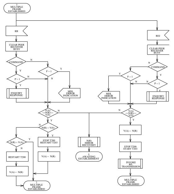
Figure 3.7-6 — Link Layer Point-to-Point: State 7, Multiple Frame Established (4 of 8)
