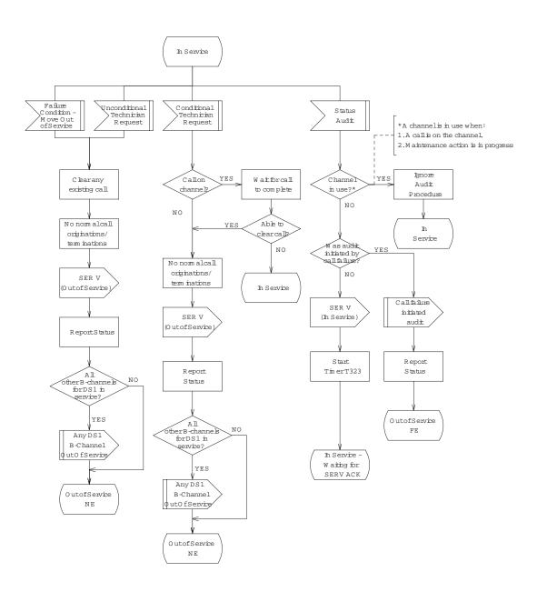
Figure 9.3-19 — National ISDN PRI with BCAS: B-channels, In Service (3 of 3)
