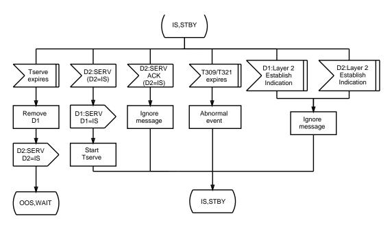
Figure 9.3-26 — National ISDN PRI with D-channel Backup: In Service, Standby (2 of 2)
