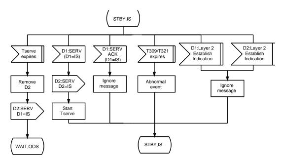
Figure 9.3-27 — National ISDN PRI with D-channel Backup: Standby, In Service (2 of 2)
