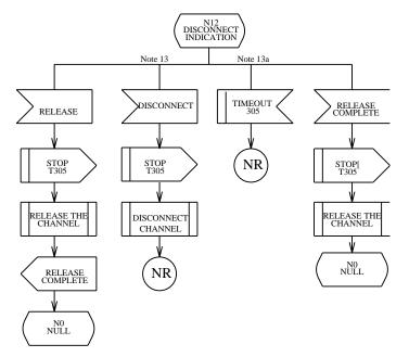
Figure 7-11 — Network Side: N12, Disconnect Indication State
