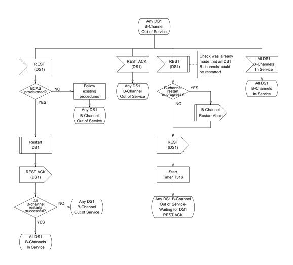
Figure 9.3-16 — National ISDN PRI with BCAS: DS1, Any B-channel Out of Service State (1 of 2)
