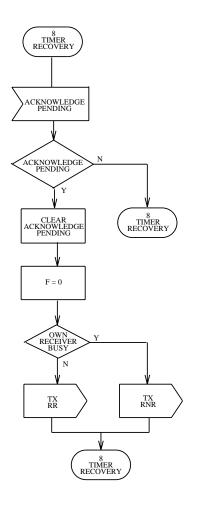
Figure 3.7-7 — Link Layer Point-to-Point: State 8, Timer Recovery (7 of 7)
