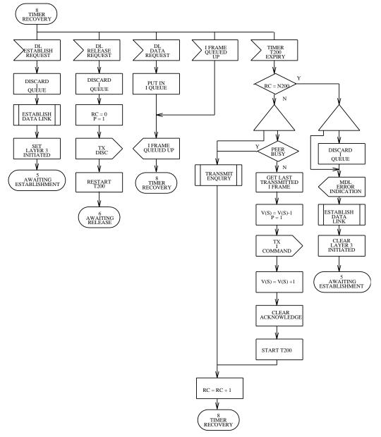
Figure 3.7-7 — Link Layer Point-to-Point: State 8, Timer Recovery (1 of 7)
