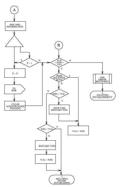
Figure 3.7-6 — Link Layer Point-to-Point: State 7, Multiple Frame Established (7 of 8)
