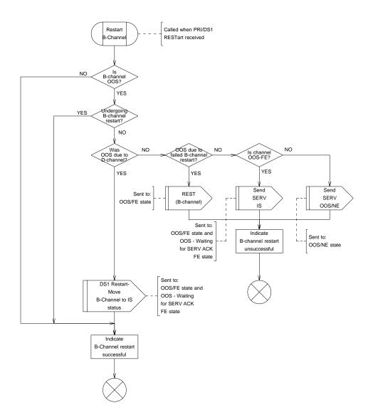
Figure 9.3-12 — National ISDN PRI with BCAS: Restart B-channel Procedure
