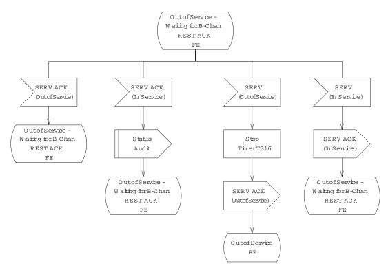
Figure 9.3-24 — National ISDN PRI with BCAS: B-channels, Out of Service FE, Waiting for B-channel REST ACK (1 of 4)
