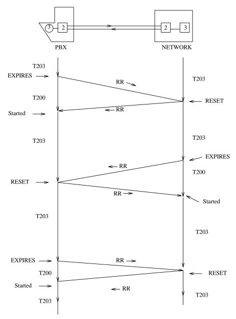
Figure 10-1 — Connection Verification Procedure on D2
