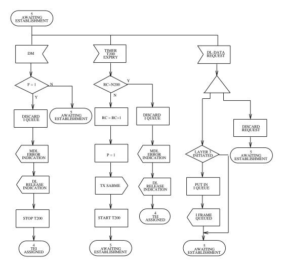
Figure 3.7-4 — Link Layer Point-to-Point: State 5, Awaiting Establishment (2 of 2)
