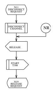
Figure 7-15 — Network Side: N11, Disconnect Request State
