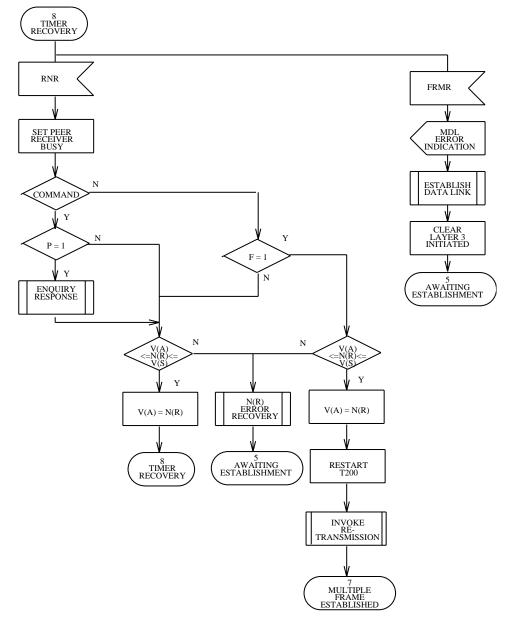
Figure 3.7-7 — Link Layer Point-to-Point: State 8, Timer Recovery (4 of 7)
