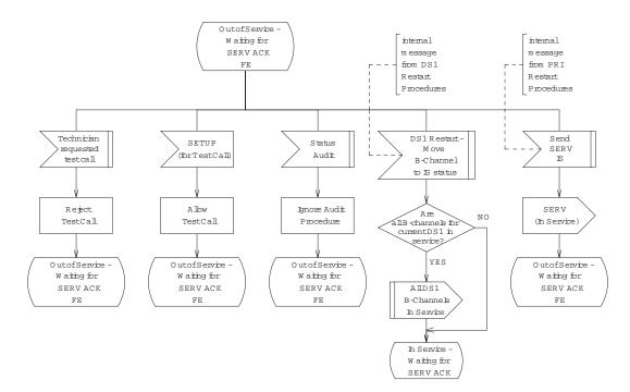
Figure 9.3-23 — National ISDN PRI with BCAS: B-channels, Out of Service FE, Waiting for SERV ACK (4 of 4)
