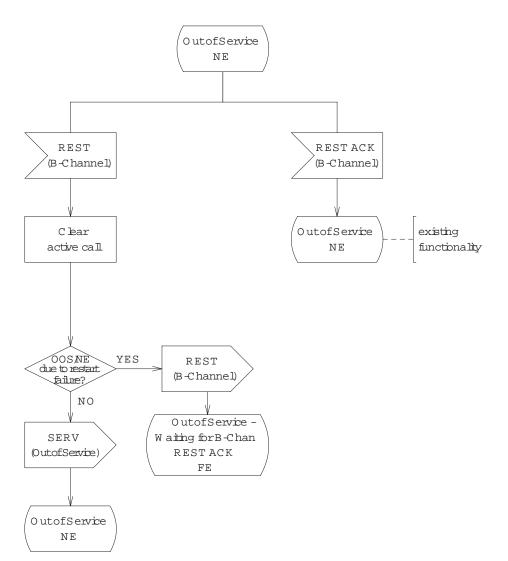
Figure 9.3-21 — National ISDN PRI with BCAS: B-channels, Out of Service NE (2 of 3)
