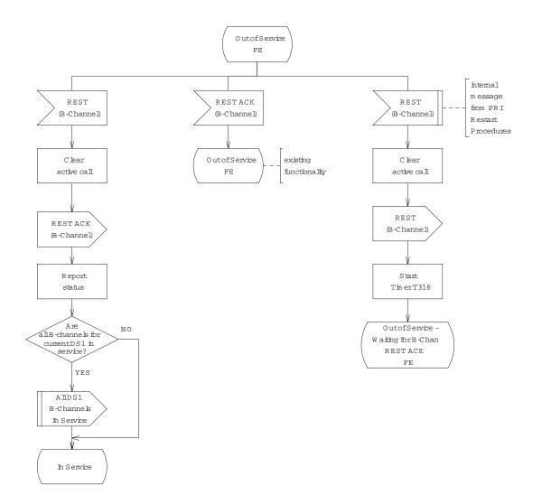
Figure 9.3-22 — National ISDN PRI with BCAS: B-channels, Out of Service FE (2 of 4)
