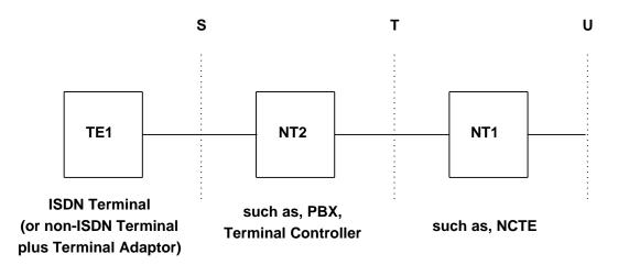
*Note:* NT1, NT2, and TE1 are functional or logical units and are not necessarily physically discrete. The reference points S, T, and U are demarcation points among the functional units. Functions may be merged within equipment. For example, the NT1 function may be absorbed within a PBX in which case there may be no physical interface at T. Likewise, the Terminal Adaption function may be provided within a PBX in which case there may be no physical interface at S.
