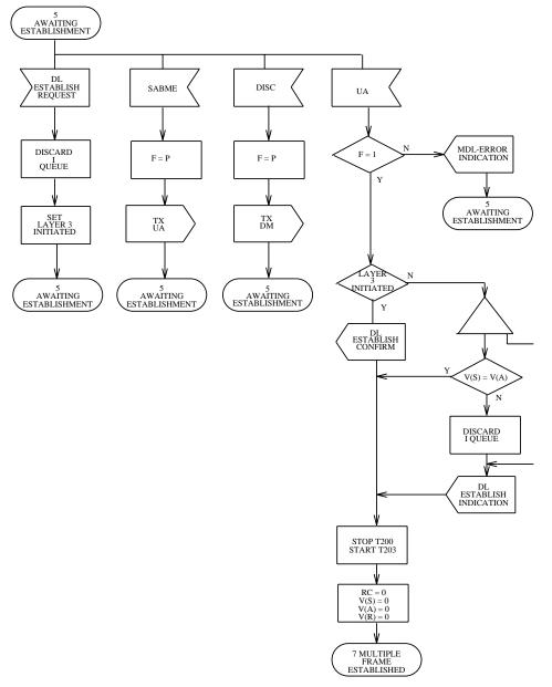
Figure 3.7-4 — Link Layer Point-to-Point: State 5, Awaiting Establishment (1 of 2)
