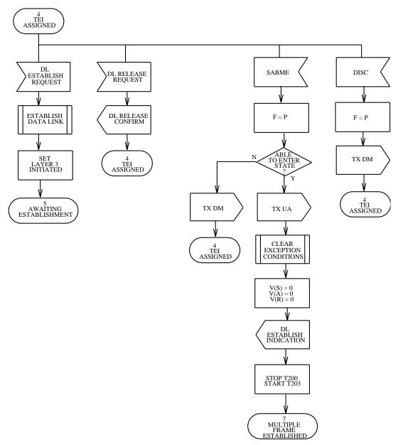
Figure 3.7-3 — Link Layer Point-to-Point: State 4, TEI Assigned (1 of 2)
