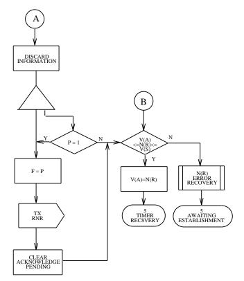
Figure 3.7-7 — Link Layer Point-to-Point: State 8, Timer Recovery (6 of 7)
