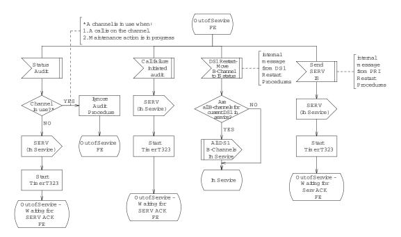
Figure 9.3-22 — National ISDN PRI with BCAS: B-channels, Out of Service FE (4 of 4)
