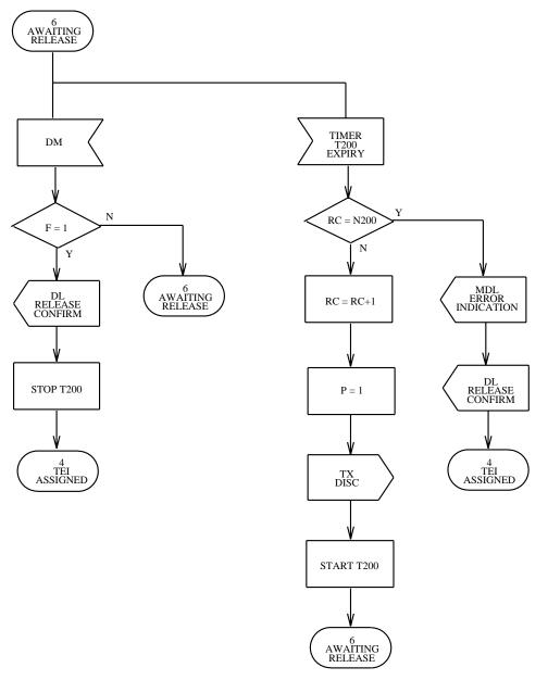
Figure 3.7-5 — Link Layer Point-to-Point: State 6, Awaiting Release (2 of 2)
