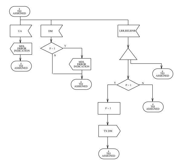
Figure 3.7-3 — Link Layer Point-to-Point: State 4, TEI Assigned (2 of 2)
