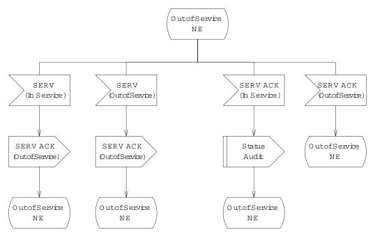
Figure 9.3-21 — National ISDN PRI with BCAS: B-channels, Out of Service NE (1 of 3)
