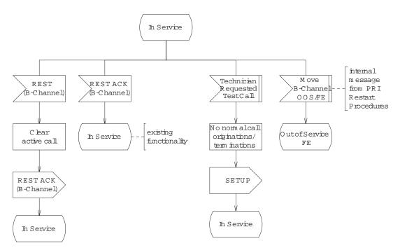
Figure 9.3-19 — National ISDN PRI with BCAS: B-channels, In Service (2 of 3)
