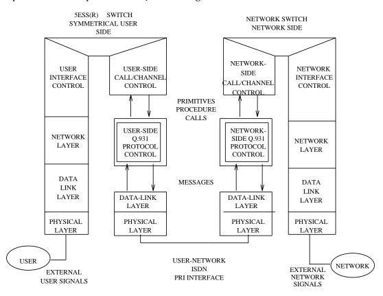
a. Protocol Stack diagram of Elements Between User and Network
