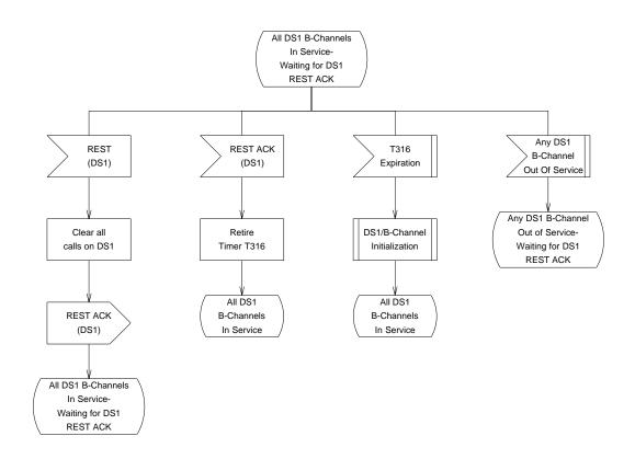
Figure 9.3-15 — National ISDN PRI with BCAS: DS1, All B-channels In Service State, Waiting for DS1 REST ACK
