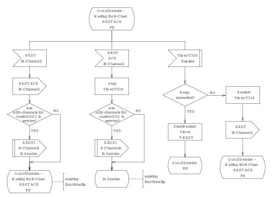
Figure 9.3-24 — National ISDN PRI with BCAS: B-channels, Out of Service FE, Waiting for B-channel REST ACK (2 of 4)
