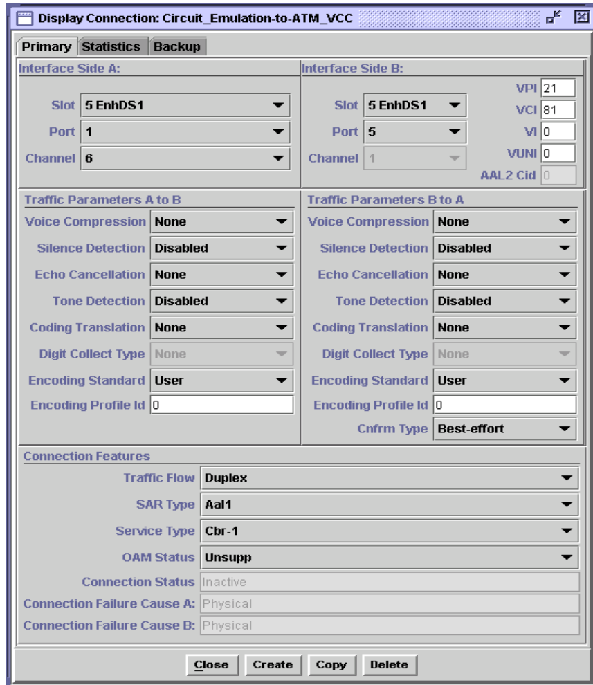
Figure 8-15. Display Connection: Circuit_Emulation-to-ATM_VCC (Primary Page)
