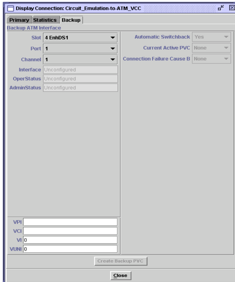
Figure 8-17. Display Connection: Circuit_Emulation-to-ATM_VCC (Backup Page)
