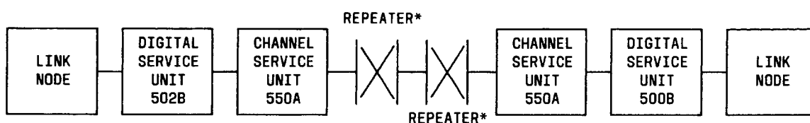
Fig. 7—Digital Signaling Link (1000 Feet or Less)
