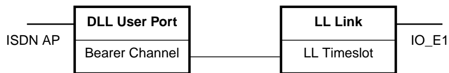
Figure 7-21 Functional model of DLL user port configuration
