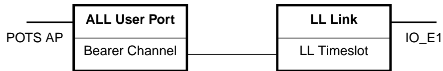
Figure 7-17 Functional model of ALL user port configuration
