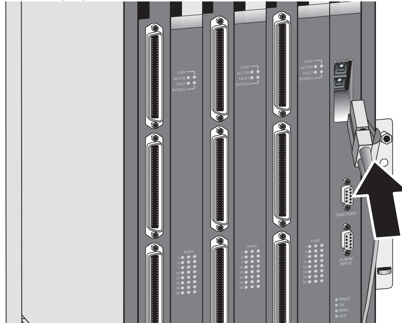
Figure 3-25. 155Mbps optical connection to the COP
