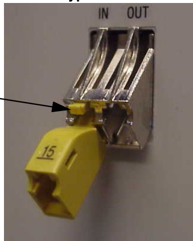
Figure C-4 Removing LC-Type LBO From LC-Type Connector Port
