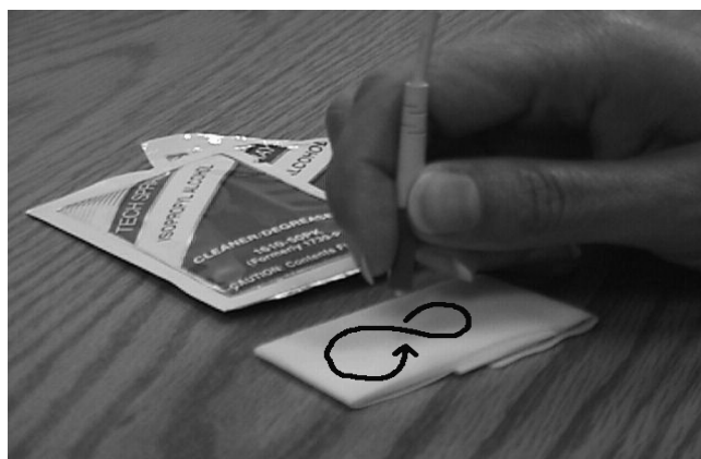
Figure B-1 Cleaning the Ferrule Endface
