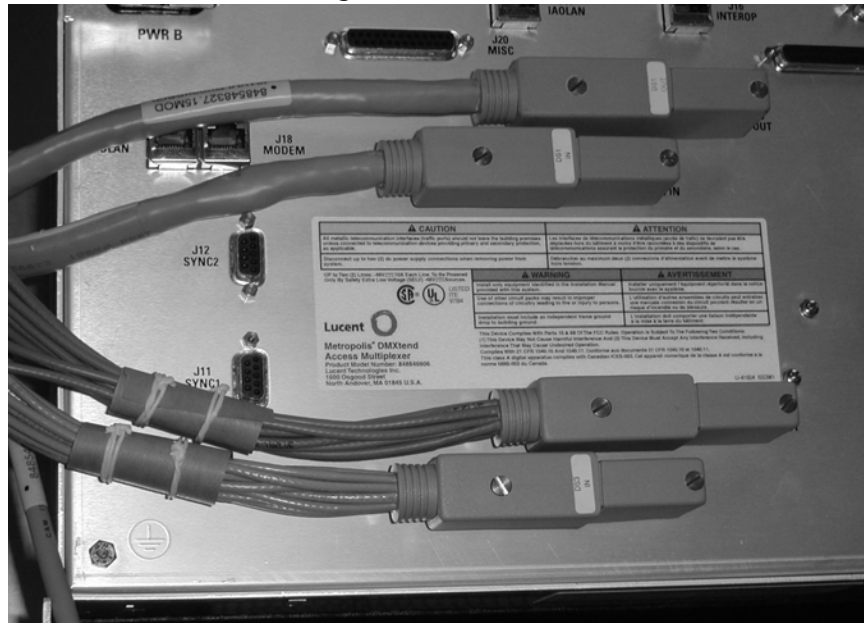
Figure 3-7 DS3/EC-1 cable routing to the left
