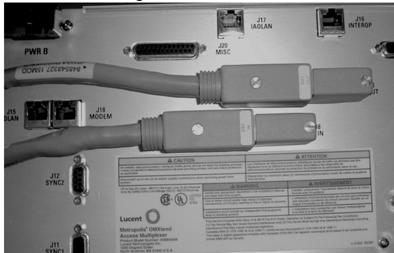
Figure 3-4 DS1/E1 cable routing to the left
