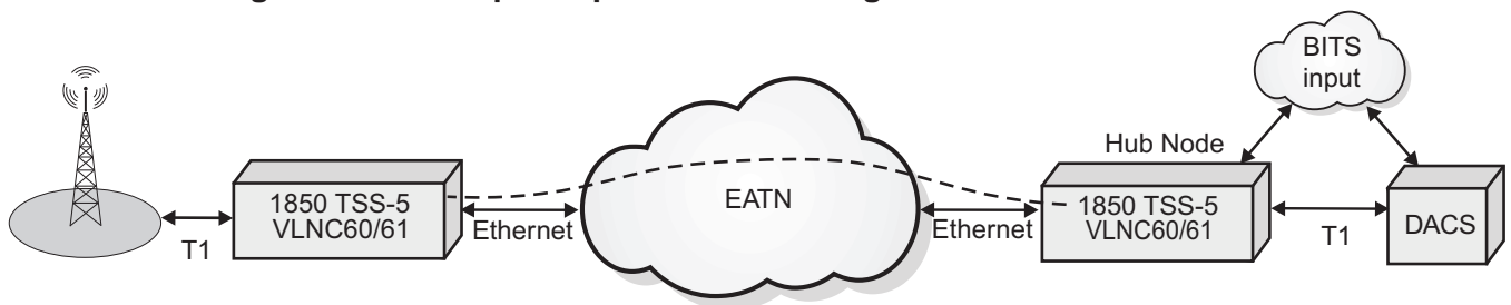
Figure A-9 Example of pseudowire timing
