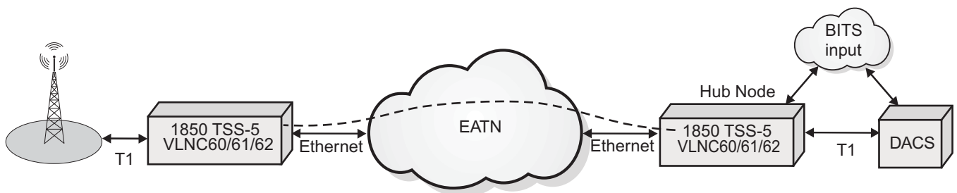
Figure A-9 Example of pseudowire timing
