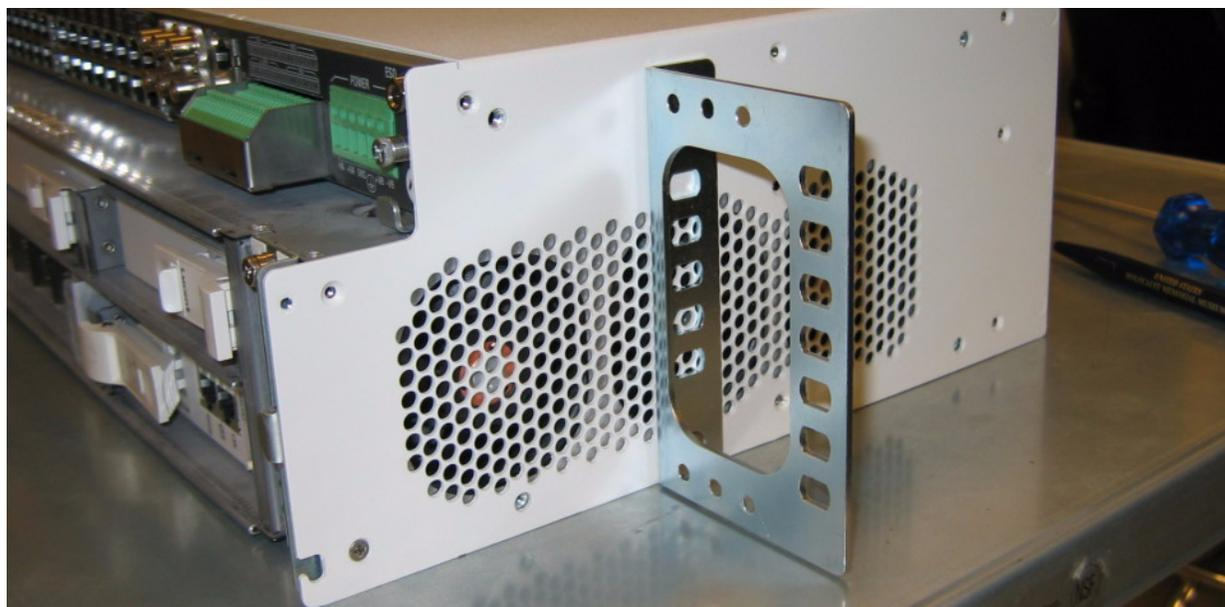
**Figure 2-7** Mounting bracket position for ETSI frame
