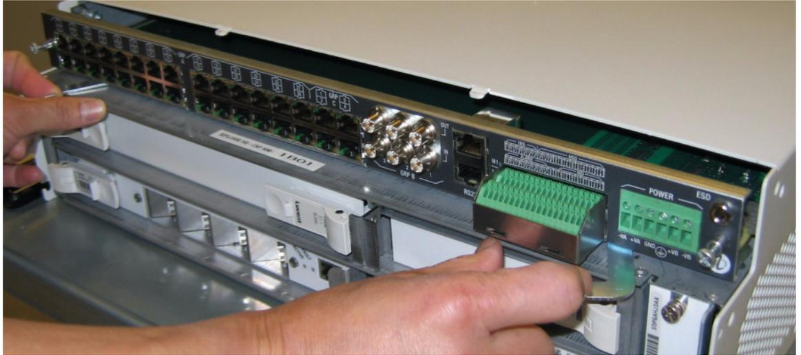
**Figure 2-2 Fully seated VLIU interface panel**
