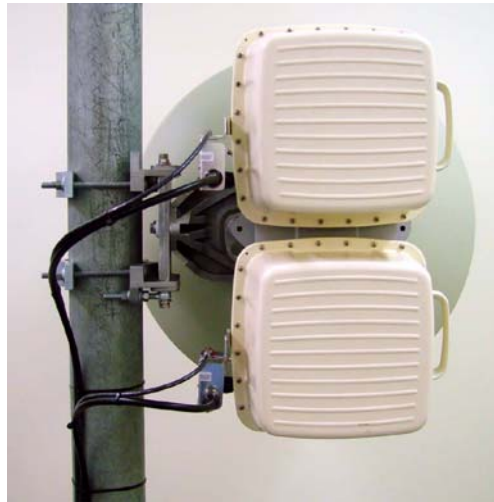
Figure 2-13. Coupler Installation with ODUs: Rear View
