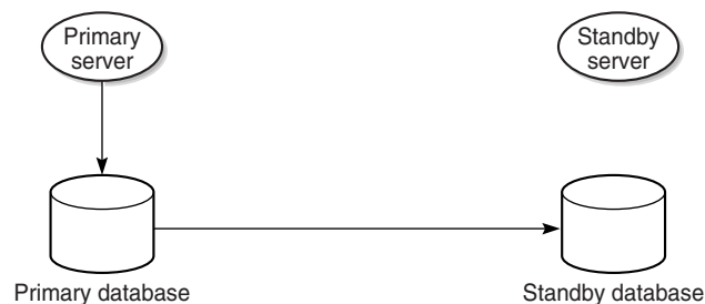
Figure 6-6 Server and database roles before database switchover
