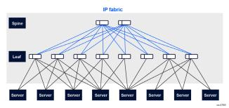
Cost, capacity, and power are also important aspects; for instance, there are multilayer switches with a higher port radix that can accommodate the newer GPU servers and can be deployed as leafs, however, these are generally more expensive and consume more power and hence are not suitable for small to medium clusters.
