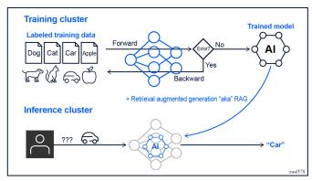
An inference cluster is used to deploy a trained model with or without reinforcements such as retrieval-augmented generation (RAG) to answer queries from the consumer based on its training data. This is less intensive than the training portions and hence has fewer infrastructure requirements.
