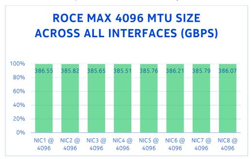
Perftest results for ib\_send\_bw showing average bi-directional bandwidth achieved across 400Gb interfaces, all using the maximum RoCE 4096-byte MTU size
