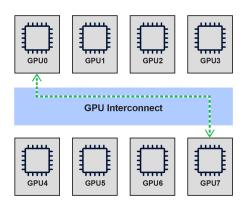
Intra-node communication refers to the communication between GPUs in a single server. We can see in the Lenovo SR 685a schema that each AMD Mi 300X GPU has full mesh connectivity to every other GPU via the internal switch.
