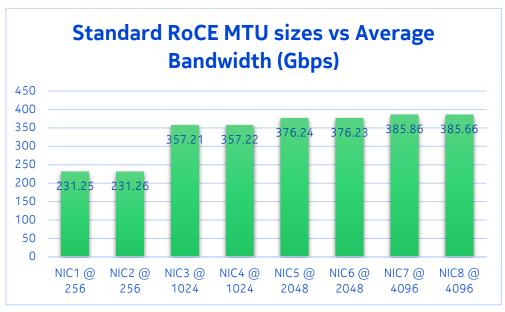
Perftest results for ib\_send\_bw showing average bi-directional bandwidth achieved across 400Gb interfaces with the standard RoCE packet sizes from 256 to 4096 bytes
