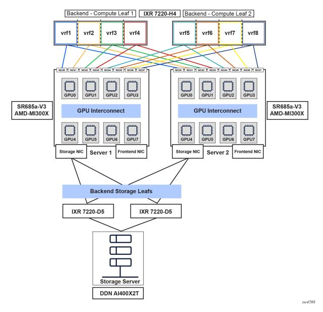
For redundancy, the storage network comprises two /25 Ethernet subnets, each one served by a storage leaf.
