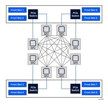
The figure shows the GPU switching reference architecture for the Lenovo SR685a GPU server capable of hosting the AMD MI300X series GPU.
