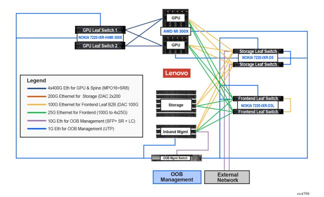
The figure above shows the Lenovo-Nokia AI validated scalable unit, which has been used as the test bed for this validated design.
