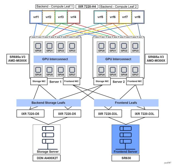
The diagram above shows the reference architecture of the Lenovo-Nokia validated design pod, which demonstrates a reduced form of a typical rail-only design achieved via IP VRFs called node isolation groups.
