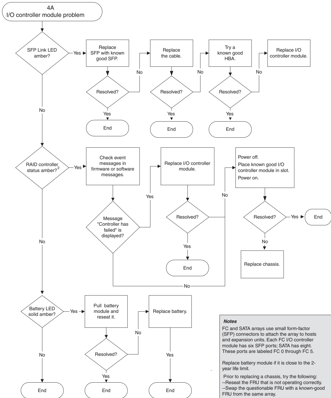
FIGURE 8-10 I/O Controller Module Flowchart
