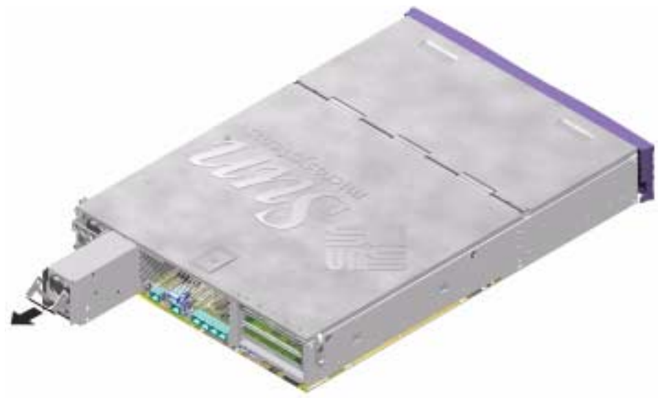
FIGURE 1-13 Removing a PSU on a Sun Fire V240 Server
