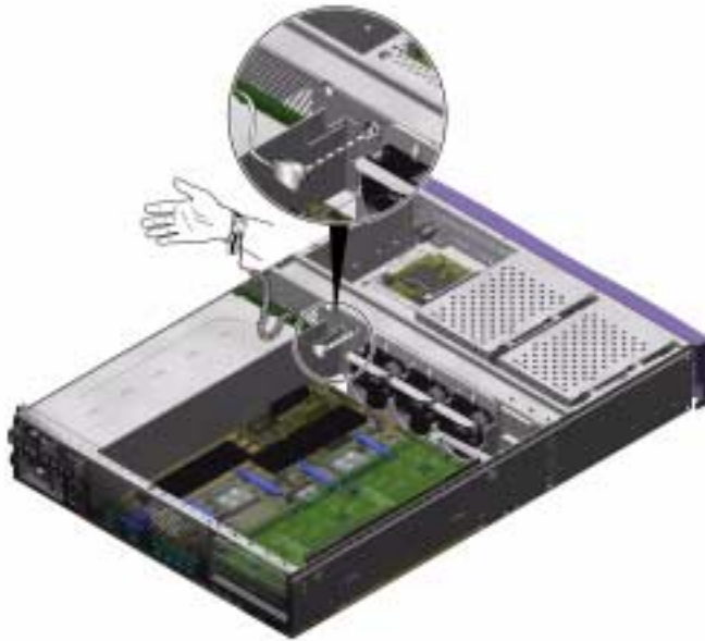
FIGURE 1-1 Grounding Point in the Back of the Servers (Sun Fire V240 shown)
