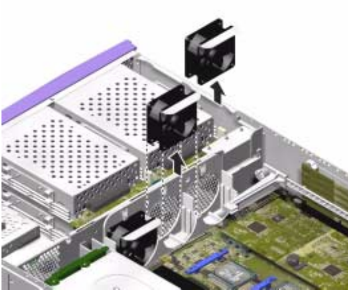
FIGURE 1-18 Removing Fans (Sun Fire V240 server shown)
