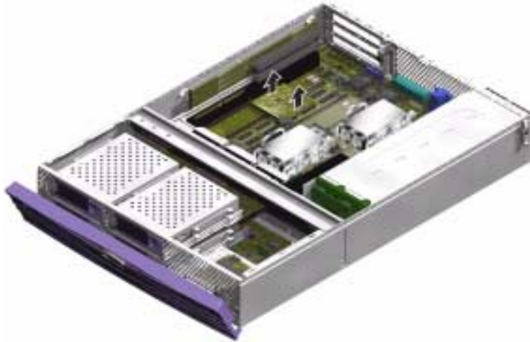
FIGURE 1-29 Removing the Hardware Cryptographic Module
