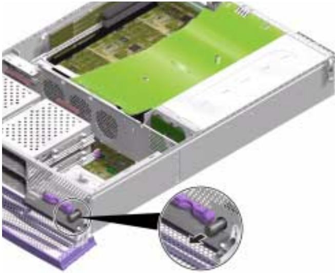
FIGURE 1-32 Removing the Keyswitch Assembly
