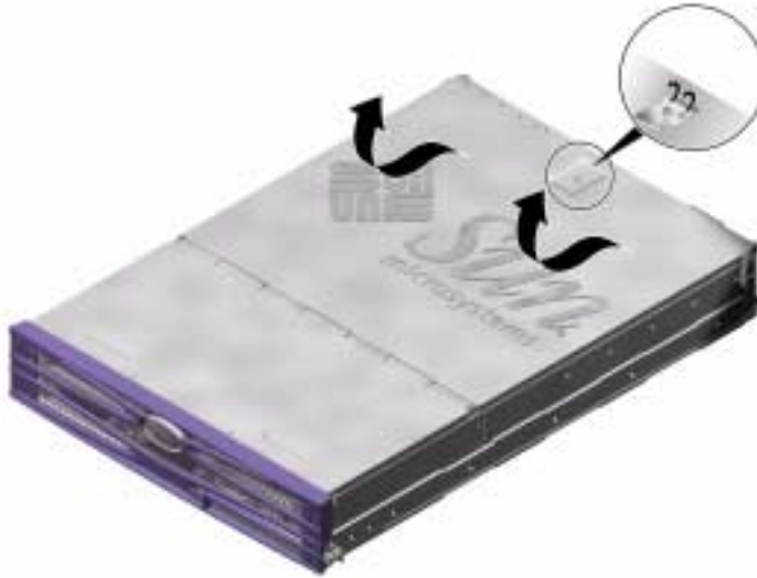
FIGURE 1-5 Location of Catch on Back Section of Lid
