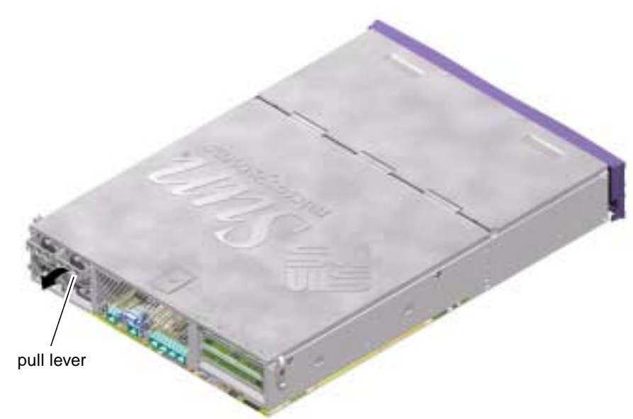
FIGURE 1-12 Power Supply Unit Lever on a Sun Fire V240 Server
