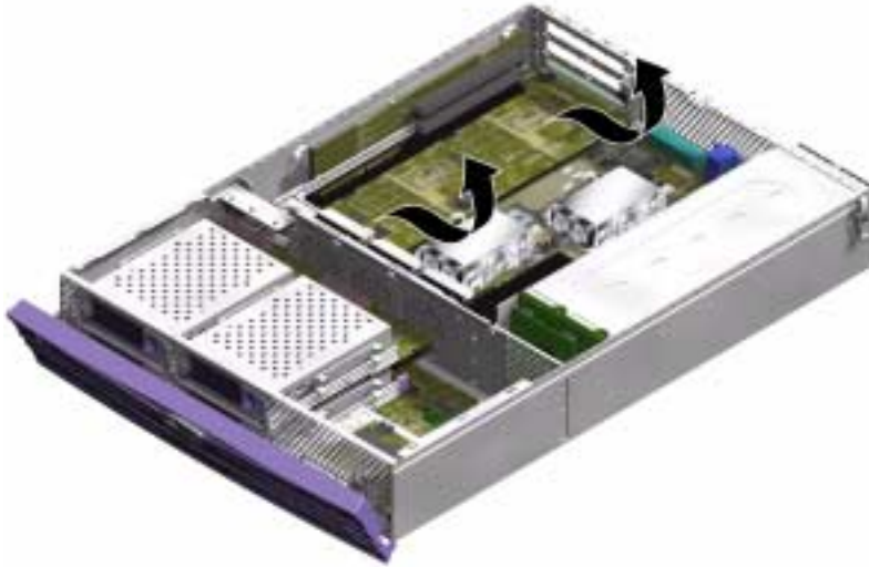
FIGURE 1-26 Removing a PCI Card on a Sun Fire V240 Server
