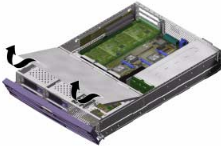
FIGURE 1-3 Removing the Front Section of the Lid
