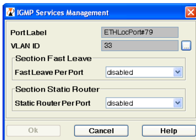
Figure 4-79 Port: IGMP Services Management
