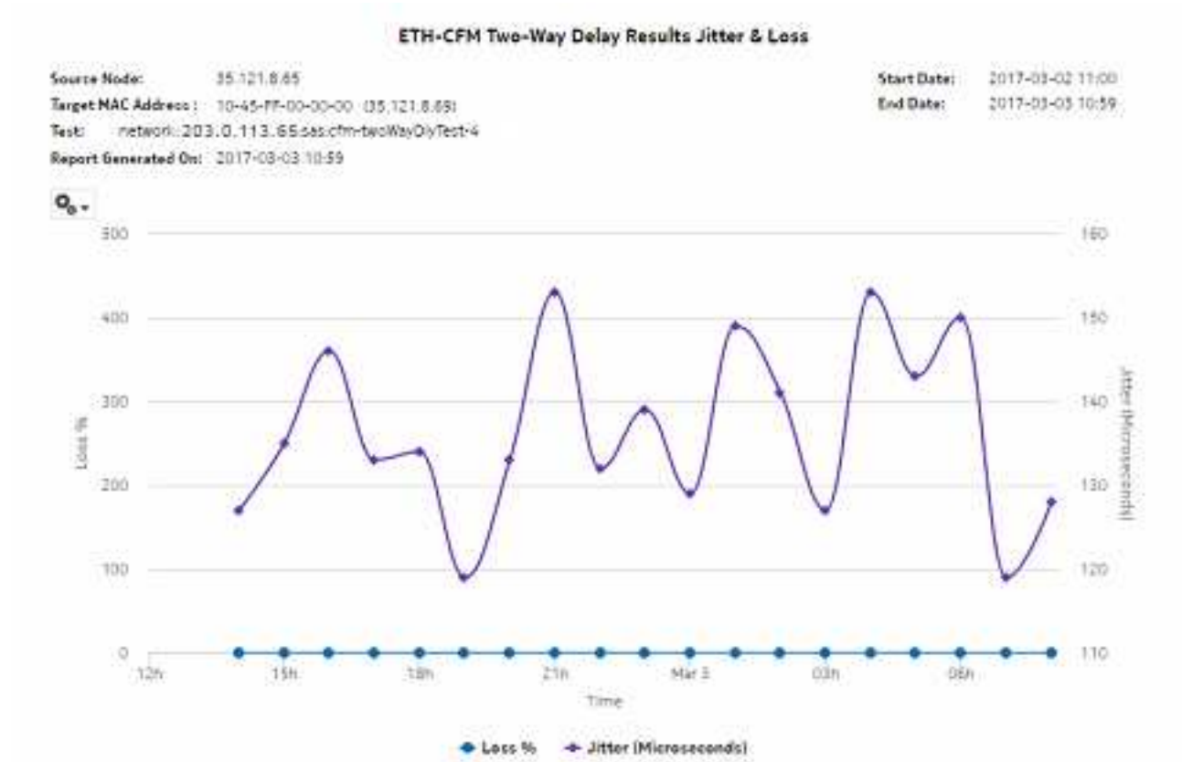
Figure 13-55 ETH-CFM Two Way Delay Results Jitter & Loss report
