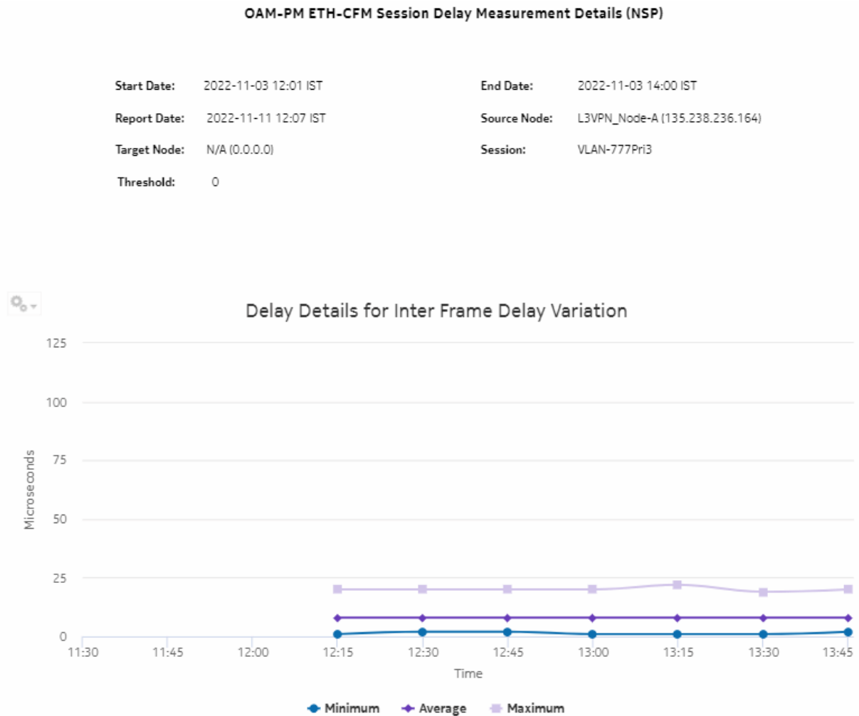
Figure 17-11 OAM-PM ETH-CFM Session Delay Measurement Details (NSP) – Delay Details for Inter Frame Delay Variation
