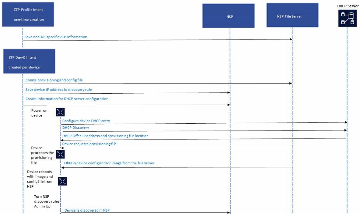
Figure 6-1 Zero Touch Provisioning process
