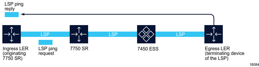
Figure 90-5 LSP ping OAM diagnostic test
