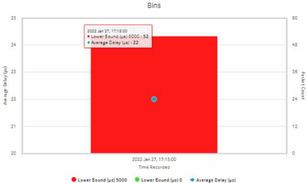
Figure 18-6 OAM-PM Bins and Delay (NSP) report – MDM NE CFM DMM light session bins and delay
