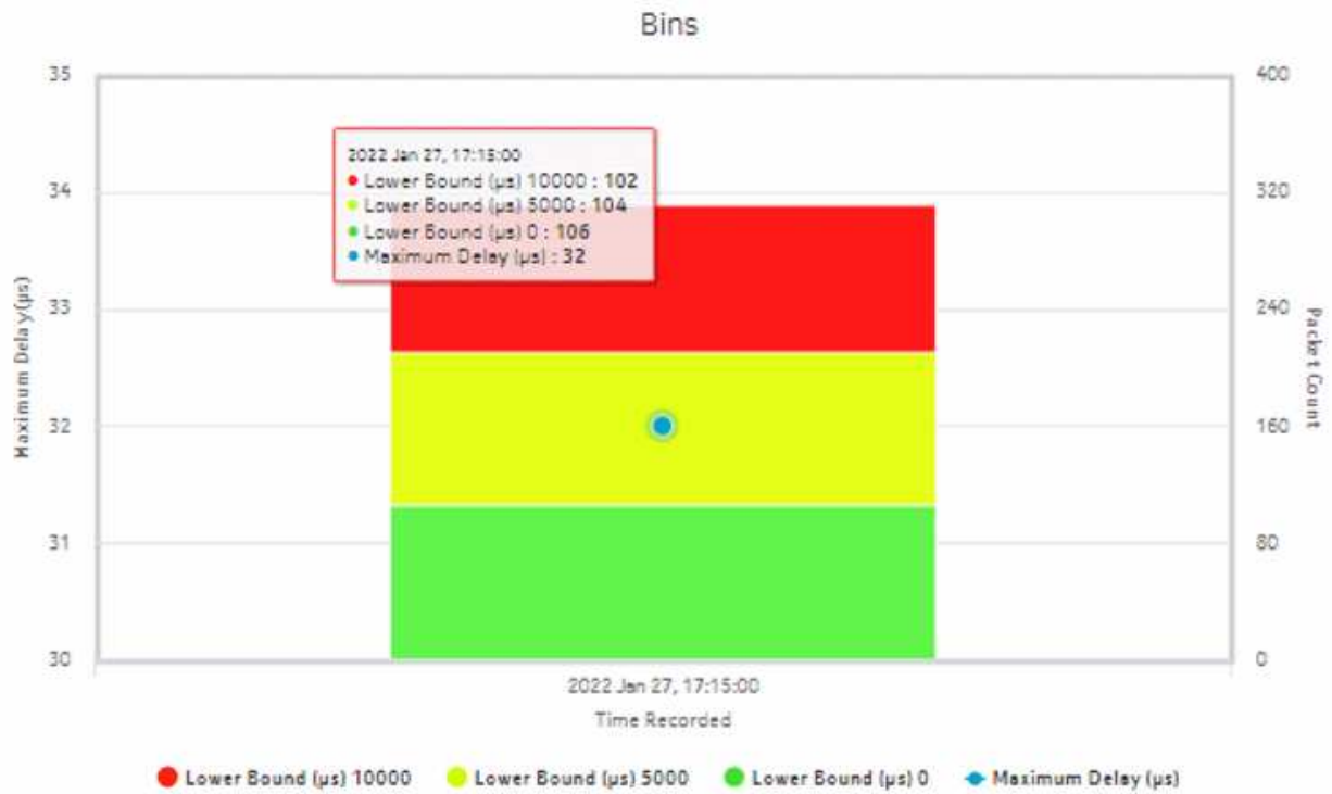
Figure 18-5 OAM-PM Bins and Delay (NSP) report – MDM NE TWAMP light session bins and delay
