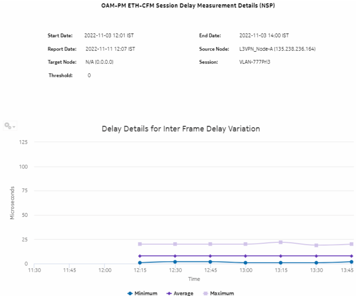
Figure 18-11 OAM-PM ETH-CFM Session Delay Measurement Details (NSP) – Delay Details for Inter Frame Delay Variation
