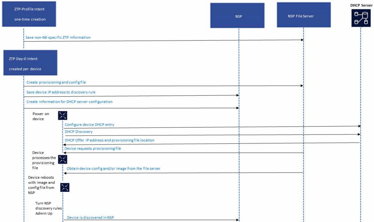
Figure 6-1 Zero Touch Provisioning process
