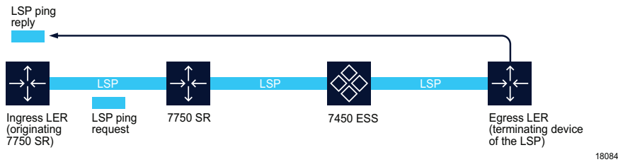
Figure 90-5 LSP ping OAM diagnostic test
