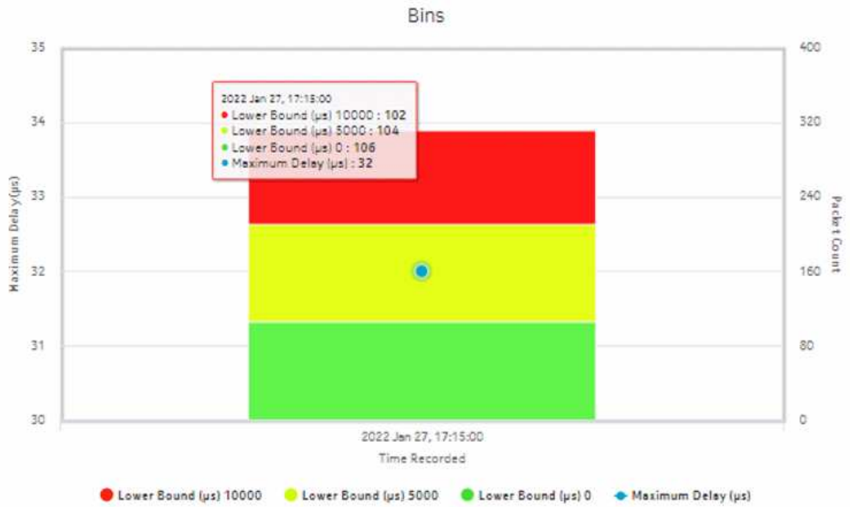
Figure 17-5 OAM-PM Bins and Delay (NSP) report – MDM NE TWAMP light session bins and delay
