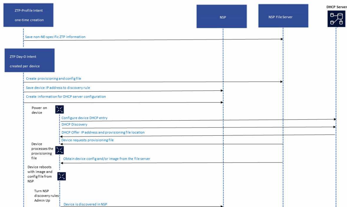
Figure 6-1 Zero Touch Provisioning process
