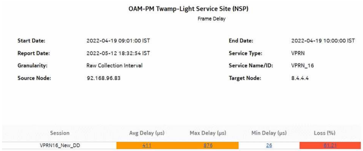
Figure 18-29 OAM-PM Twamp-Light Service Site (NSP) – Frame Delay
