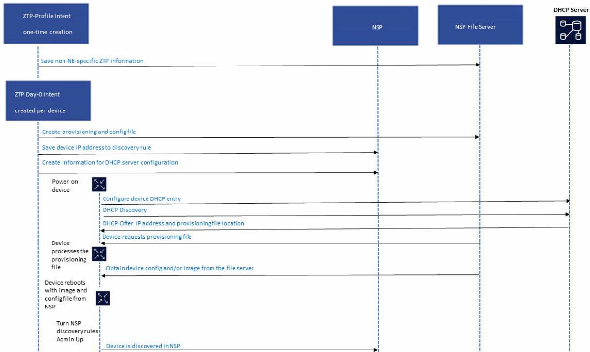
Figure 6-1 Zero Touch Provisioning process
