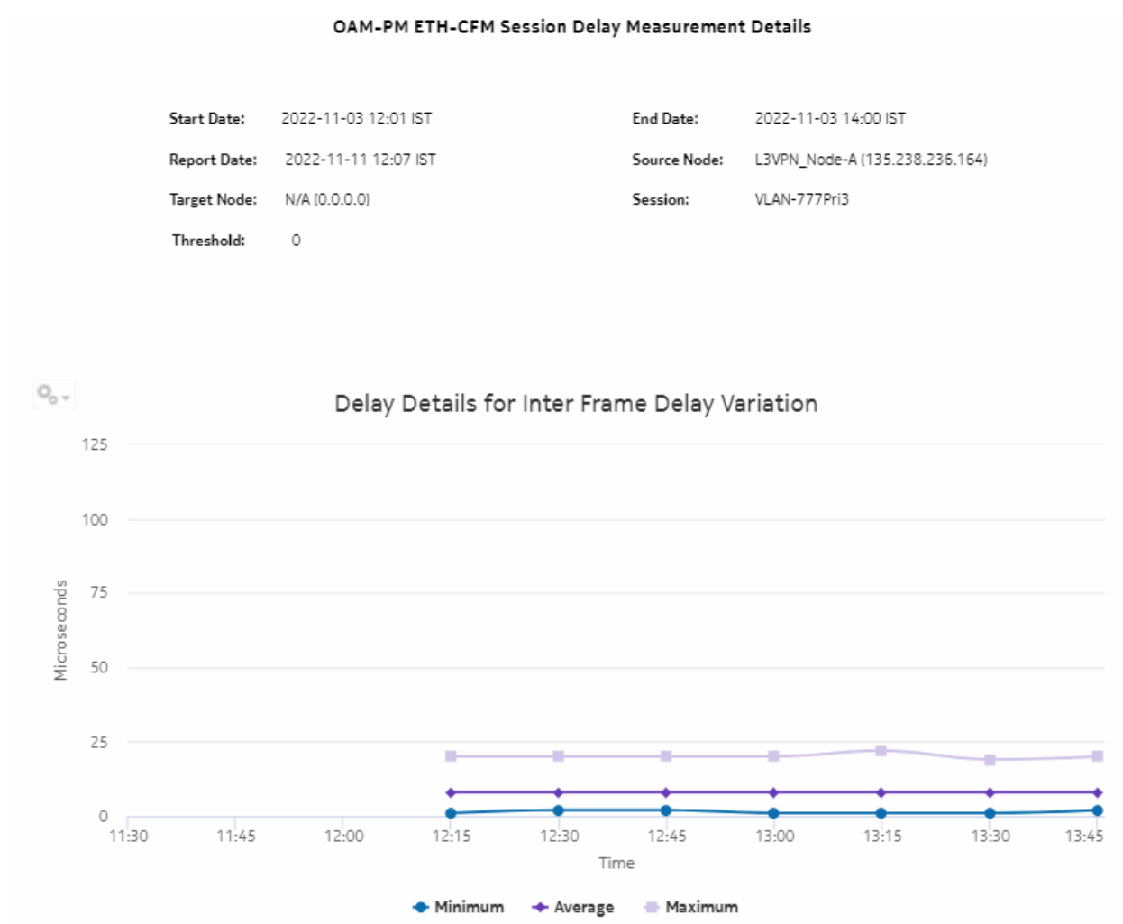
Figure 10-11 OAM-PM ETH-CFM Session Delay Measurement Details – Delay Details for Inter Frame Delay Variation
