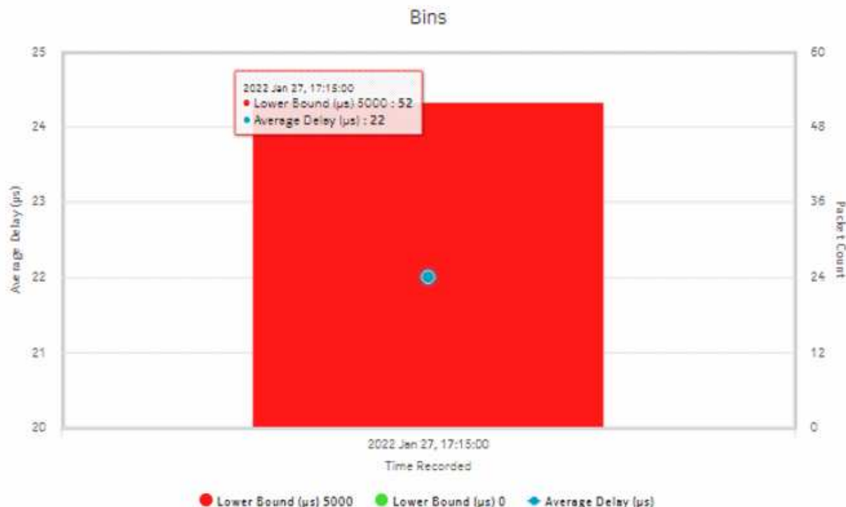
Figure 10-6 OAM-PM Bins and Delay report – MDM NE CFM DMM light session bins and delay
