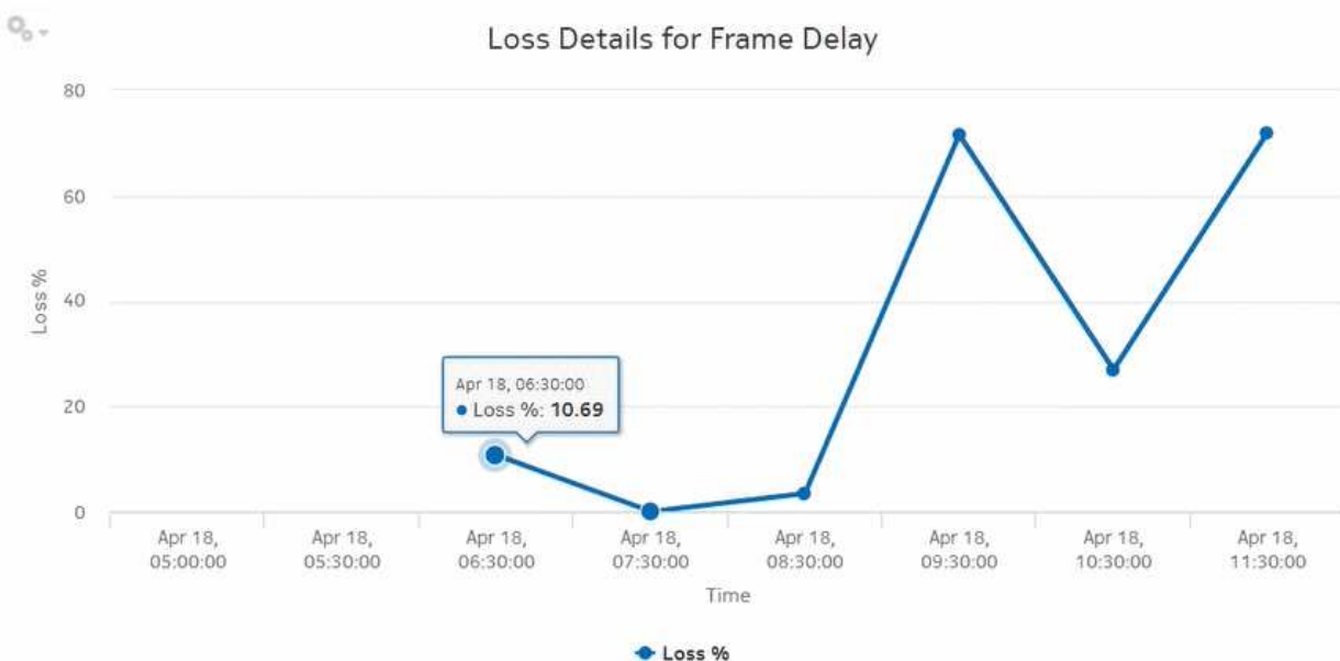
Figure 10-14 OAM-PM ETH-CFM Loss Measurement Details report – Loss Details for Frame Delay
