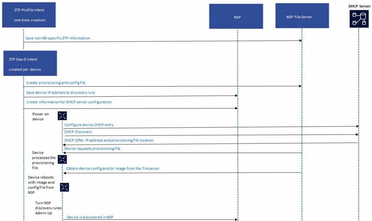
Figure 6-1 Zero Touch Provisioning process
