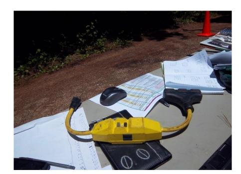
GFCI (Ground Fault Circuit Interrupter)
