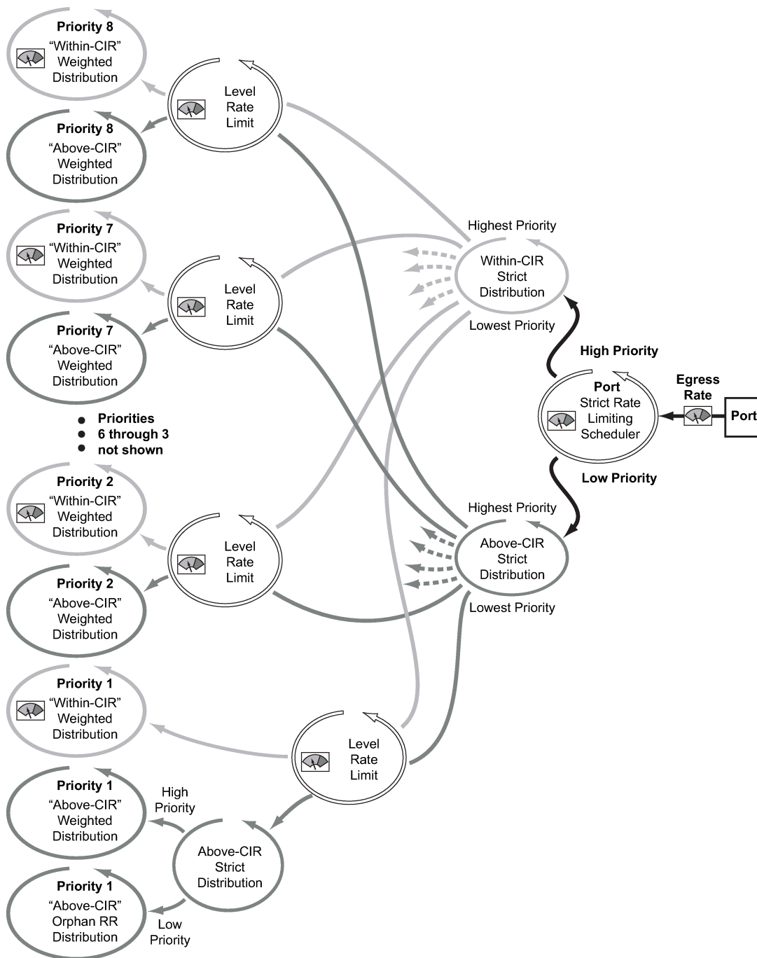
Figure 16: Port-level virtual scheduler bandwidth allocation based on priority and CIR
