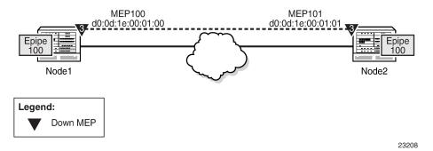
Node1 is tested for this example. The SAA configuration does not include the accounting policy required to collect the statistics before they are overwritten. Node2 does not have an SAA configuration. Node2 includes the configuration to build the MEP in the Epipe service context.
