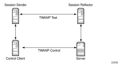
The control client and session sender are typically implemented in one physical device (also known as the client device) and the server and session reflector are typically implemented in a second physical device (also known as the server device), as shown in Figure 2: Typical TWAMP Implementation.
