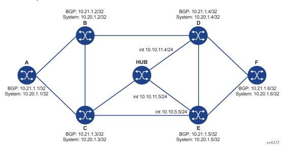
Figure 14: Topology Example for BGP Over SR-ISIS in Inter-AS Option C and BGP Over SR-TE (ISIS) in Inter-AS Option C
