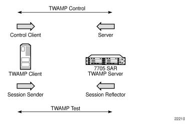
The 7705 SAR plays a passive role: the TWAMP control client initiates the control session with the 7705 SAR in order to negotiate the following:
