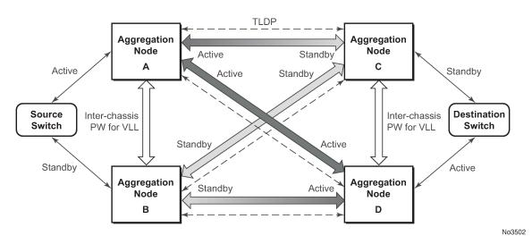
Figure 33: State Engine for Redundant Service to a Redundant Mirror Service
