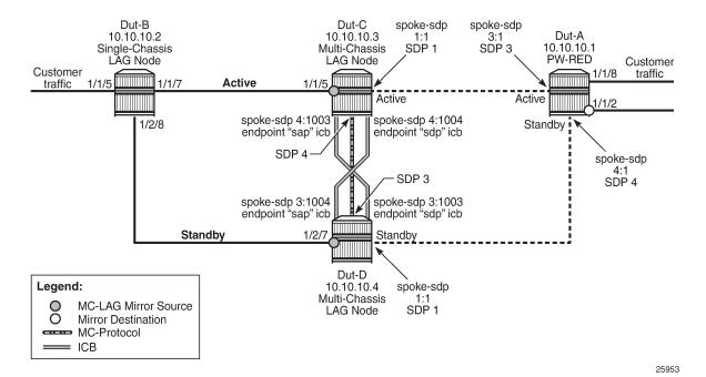
ICB spoke SDPs have been supported for Epipe services in an MC-LAG configuration. ICB spoke SDP improves switch times, provides additional protection in case of network failures, and reduces packet loss when an active endpoint is switched from a failed MC-LAG node to a protection node.
