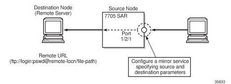
The PCAP feature supports only mirror destinations that have remote file URLs. As shown in Figure 29: PCAP Mirroring Service, the remote URL includes the absolute path and filename for the remote FTP server.
