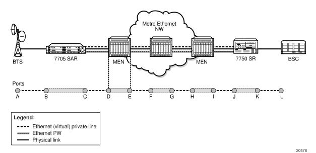
In Figure 23: EFM OAM (Dot3ah) Capabilities on the 7705 SAR, EFM OAM ensures transport layer connectivity between two directly connected nodes. Figure 23: EFM OAM (Dot3ah) Capabilities on the 7705 SAR illustrates three scenarios in which EFM can be used by the MEN provider to ensure error-free connectivity to the 7705 SAR (the cell site) via loopback tests, including:
