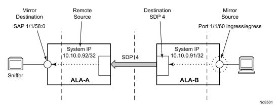
The following example shows the CLI output for configuration of remote mirrored service 1216. The traffic ingressing and egressing port 1/1/60 on 10.10.0.92 (SAR-2) will be mirrored to the destination SAP 1/1/58:0 on SAR-1.
