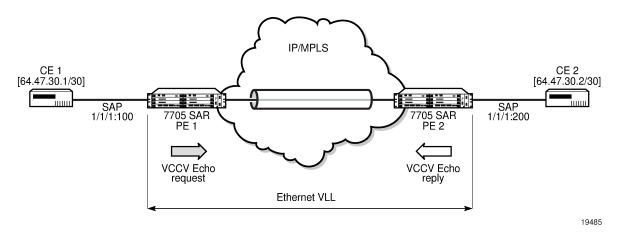
VCCV-based pseudowire (PW) tests are only supported on dynamically signaled PWs (not on statically signaled PWs).
