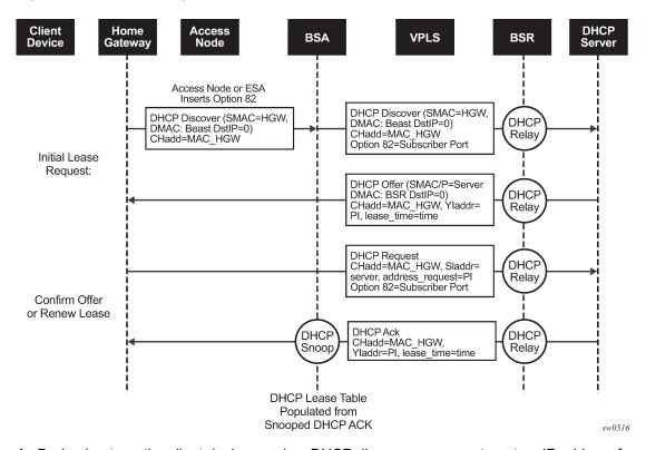
Figure 3: IP address assignment with DHCP
