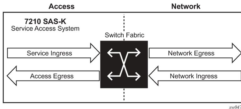
The 7210 SAS uses QoS policies applied to a SAP for a service or to an access uplink port or to a network port to define the queuing, queue attributes, meter attributes, and QoS marking/interpretation.
