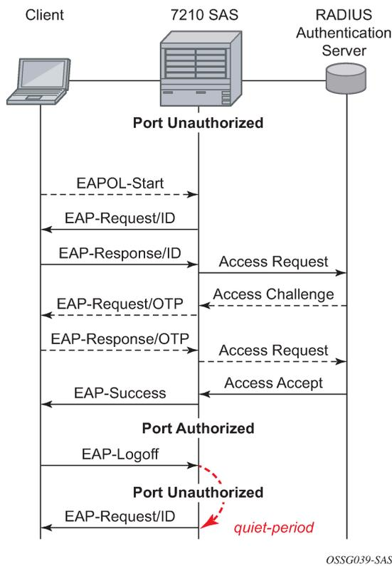
The router will initiate the procedure when the Ethernet port becomes operationally up, by sending a special PDU called EAP-Request/ID to the client. The client can also initiate the exchange by sending an EAPOL-start PDU, if it does not receive the EAP-Request/ID frame during bootup. The client responds on the EAP-Request/ID with a EAP-Response/ID frame, containing its identity (typically username + password).
