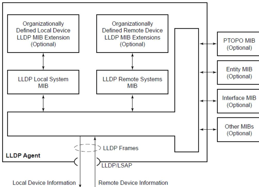
To detect and address network problems and inconsistencies in the configuration, the network operators can discover the topology information using LLDP. The Standard-based tools address the complex network scenarios where multiple devices from different vendors are interconnected using Ethernet interfaces.
