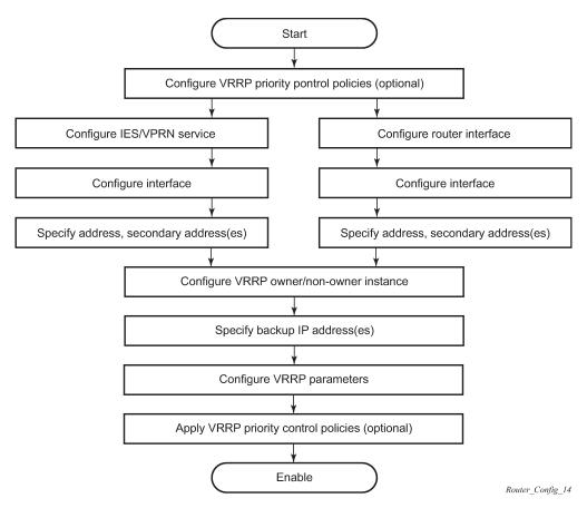
Figure 8: VRRP configuration and implementation flow
