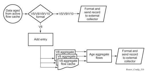
As flows expire and are removed from the active flow cache, the export format is determined (either Version 5, Version 8, Version 9, and Version 10 record format) and one of the following processes occurs:
