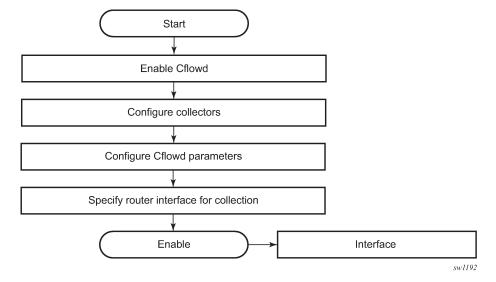
Cflowd can be enabled to sample traffic on a specific interface in the cflowd interface mode. In this mode, all traffic entering a specific port is subject to sampling as the configured sampling rate.
