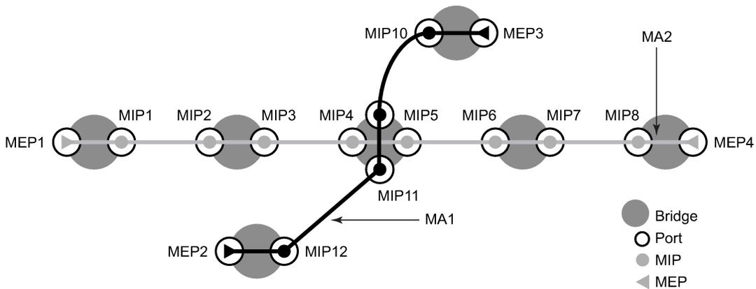
**Figure 41: MEP creation** illustrates the usage of an Epipe on two different nodes that are connected using ether SAP 1/1/2:100.31. The SAP 1/1/10:100.31 is an access port that is not used to connect the two nodes.
