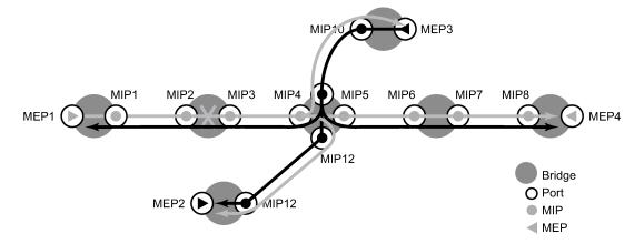
Figure 48: CFM CC failure scenario
