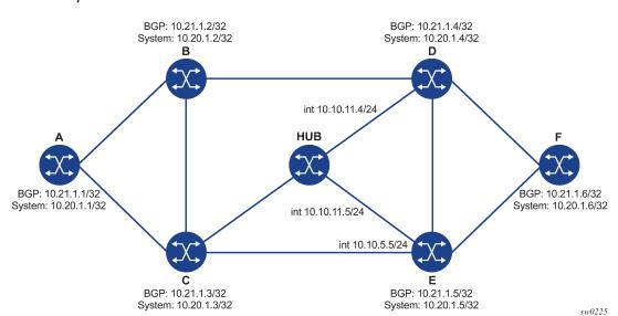
Figure 29: Example topology for BGP over SR-ISIS in inter-AS option C and BGP over SR-TE (ISIS) in inter-AS option C
