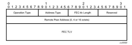
The operation type specifies the action associated with the FEC stack change. The following operation types are defined.
