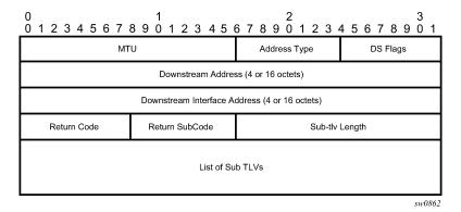
The DDMAP TLV format is derived from the DSMAP TLV format. The key change is that variable length and optional fields have been converted into sub-TLVs. The fields have the same use and meaning as in RFC 8029 as shown in Figure 22: FEC stack change sub-TLV.
