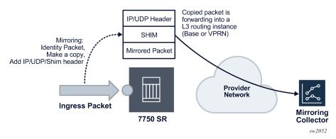
Figure 4: Shim header format
