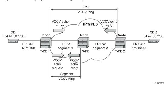
Figure 39: VCCV ping over a multi-segment pseudowire
