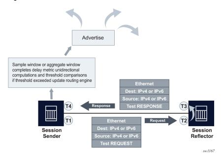
This process can also operate in a reporting disabled mode using the **configure test-oam link-measurement measurement-template reporting** command. In this mode, all processes continue to operate, including threshold comparisons. In the reporting disabled mode, the routing engine is not made aware of the threshold event.
