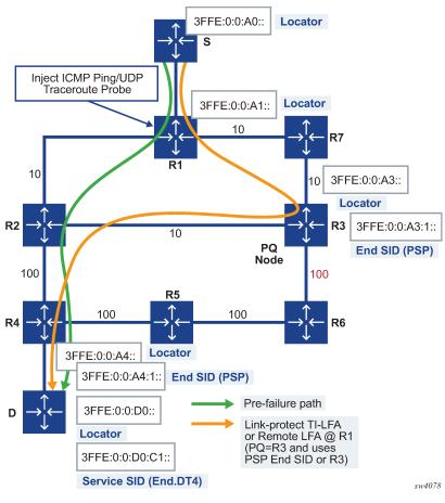
Figure 32: SRv6 OAM network setup
