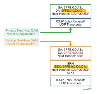
The outer IPv6 header hop-limit field is set according to the operation of the probe. For ping, the hop limit uses the default 254 or a user-entered value.
