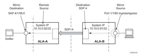
The following example shows the CLI output showing the configuration of remote mirrored service 1216. The traffic ingressing and egressing port 1/1/60 on 10.10.0.92 (ALA-B) is mirrored to the destination SAP 1/1/58:0 on ALA-A.
