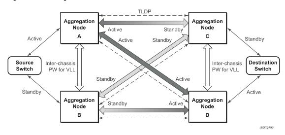
Figure 19: State engine for redundant service to a redundant mirror service
