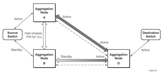
Figure 11: State engine for redundant service to a non-redundant mirror service
