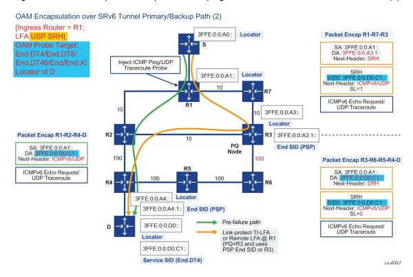
Figure 35: End-to-end packet encapsulation for ping or traceroute of a remote locator or SID (2)
