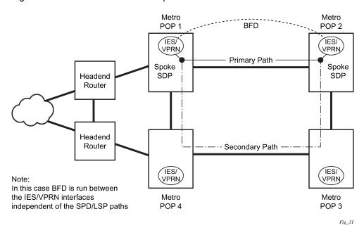
Figure 54: BFD for IES/VPRN over spoke SDP
