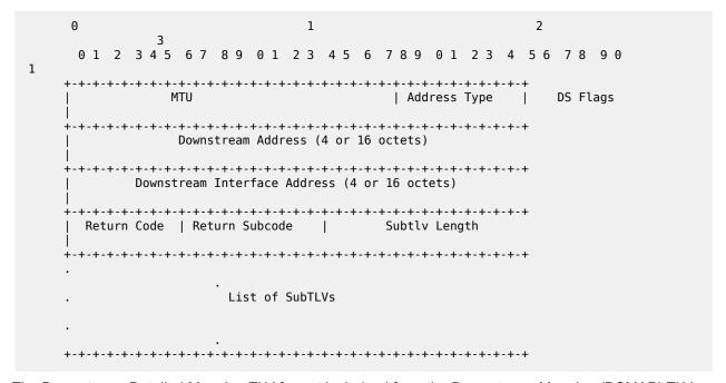
The Downstream Detailed Mapping TLV format is derived from the Downstream Mapping (DSMAP) TLV format. The key change is that variable length and optional fields have been converted into sub-TLVs. The fields have the same use and meaning as in RFC 8029.
