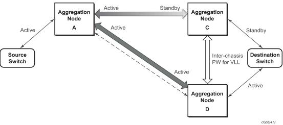
In the case where a non-redundant service is being mirrored to a redundant mirror service (Figure 12: State engine for a non-redundant service to a redundant mirror service) the source aggregation node (A) can only maintain a pseudo wire to the active destination aggregation node (D). Should the link between aggregation node D and the destination switch fail then the pseudo wire must switch to the new active aggregation node (C).
