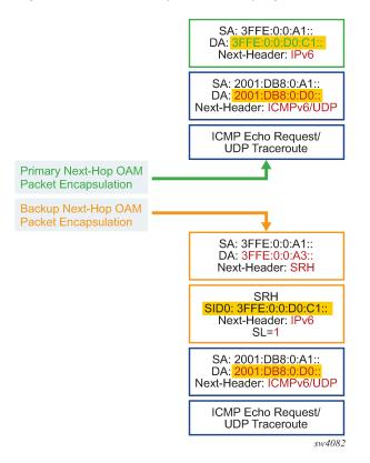
Figure 36: Packet encapsulation for ping or traceroute of a VRF IPv6 prefix over an SRv6 tunnel
