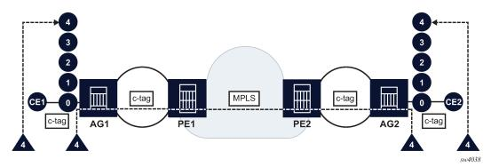
Two different squelch functions are supported, using the **squelch-ingress-levels** command and the **squelch-ingress-ctag-levels** command.
