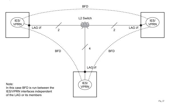
Figure 55: BFD over LAG and VSM interfaces
