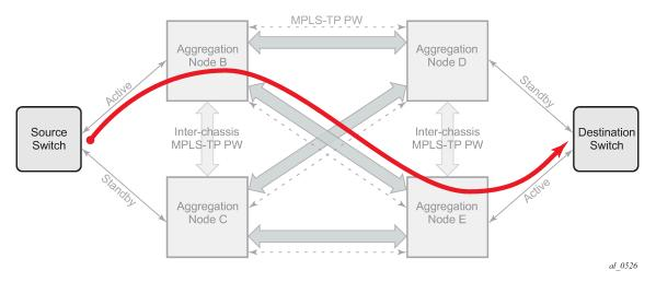
Note that mirroring traffic is usually unidirectional, flowing from "source" nodes (B or C) to "destination" nodes (D or E). However, in case of MPLS-TP, the control channel status packets may flow in the reverse direction.
