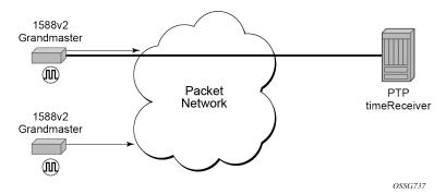
The PTP timeReceiver capability is implemented on the CPM, version 3 or later. The IEEE 1588v2 messages can ingress and egress the router on any line interface. Figure 21: Ordinary timeReceiver clock operation shows the operation of an ordinary PTP clock in timeReceiver mode.
