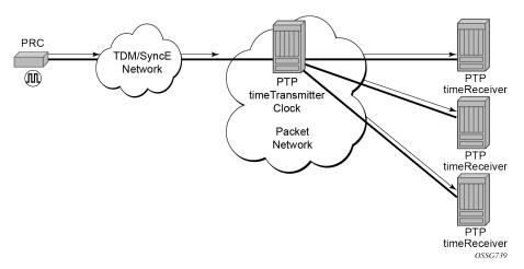
All packets are routed to their destination via the best route as determined in the route table; see Figure 23: Ordinary timeTransmitter clock operation. It does not matter which ports are used to ingress and egress these packets (unless port based time stamping is enabled for higher performance).
