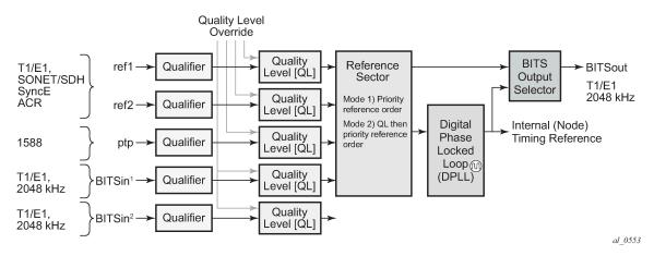
Figure 14: CPM clock synchronization reference selection
