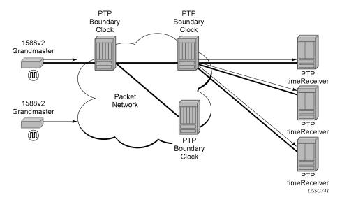
In addition, the use of port-based timestamping in every network element between the grandmaster and the end timeReceiver application is highly recommended for delivering time to meet one microsecond accuracies required of mobile applications.
