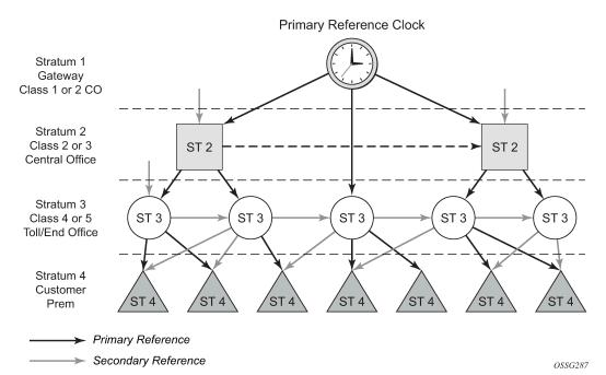
Figure 13: Conventional network timing architecture (North American nomenclature)
