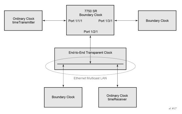
The ordinary clock timeTransmitter, ordinary clock timeReceiver, and boundary clock allow for PTP operation over both unicast IPv4 and multicast Ethernet at the same time.
