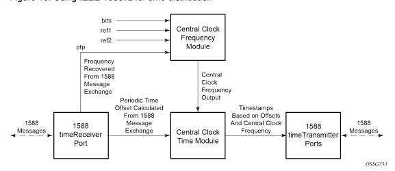
Figure 19: Using IEEE 1588v2 for time distribution
