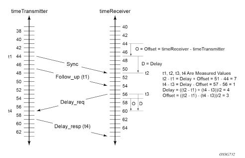
Figure 18: PTP timeReceiver and timeTransmitter time synchronization computation
