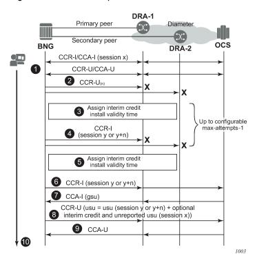
Figure 201: EFH - example call flow shows a sample call flow with EFH enabled. The following describes the call flow.
