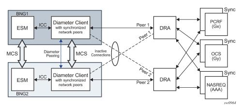
Figure 230: Multi-chassis redundancy in DRA environment
