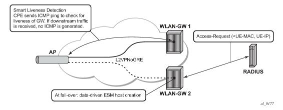
Figure 169: Inter WLAN-GW mobility based on data-triggered authentication and subscriber creation
