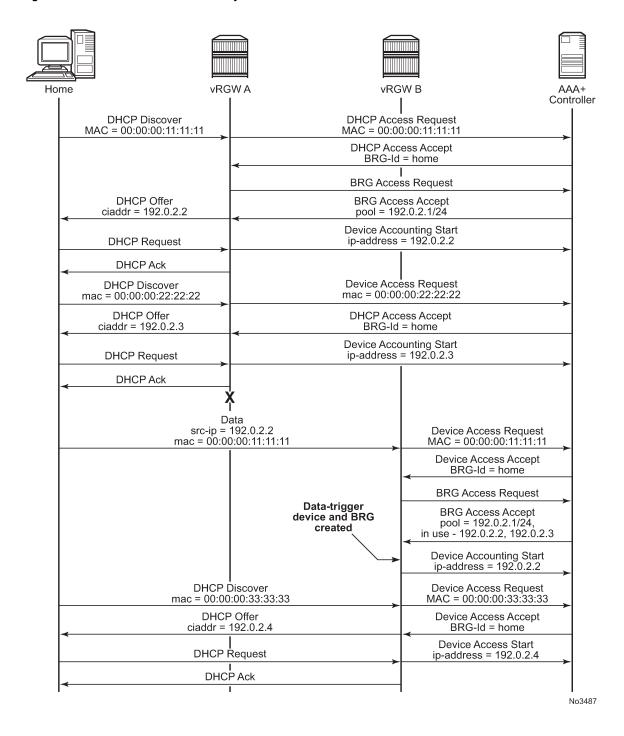
Figure 187: Inter-chassis redundancy
