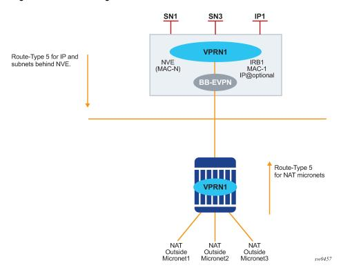
Figure 193: NVE routing traffic to and from the SF
