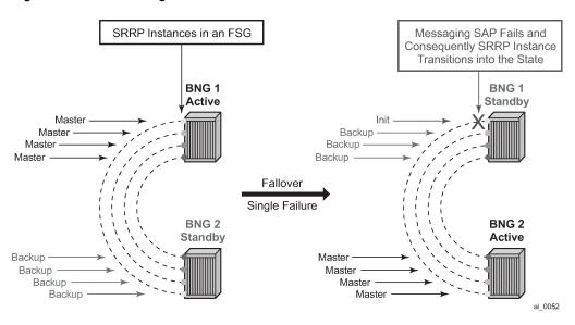
Figure 112: FSG — single network failure
