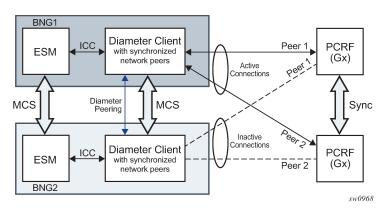
Figure 234: Collocated peer connections
