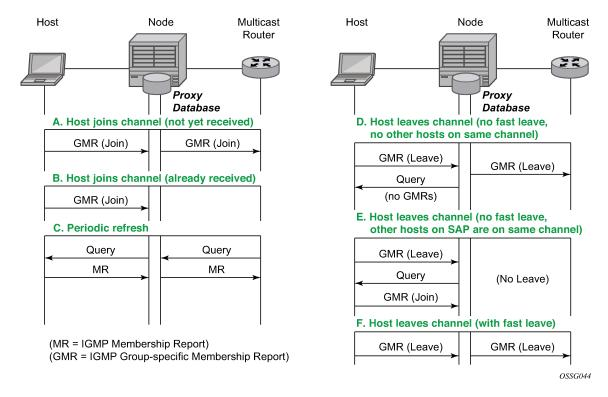
Figure 52: IGMP/MLD message processing
