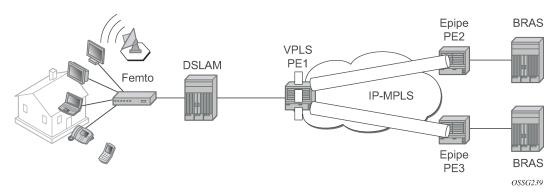
Figure 6: Subnetting topology displays a Layer 2 PE network (such as the ESS-Series) aggregating traffic from DSLAMs (Nokia) to BRAS devices. The VPLS service is running in the PEs directly connected to the DSLAMs (VPLS PE1) while the PEs connected to the BRAS devices are running a point-to-point Layer 2 service (Epipe).
