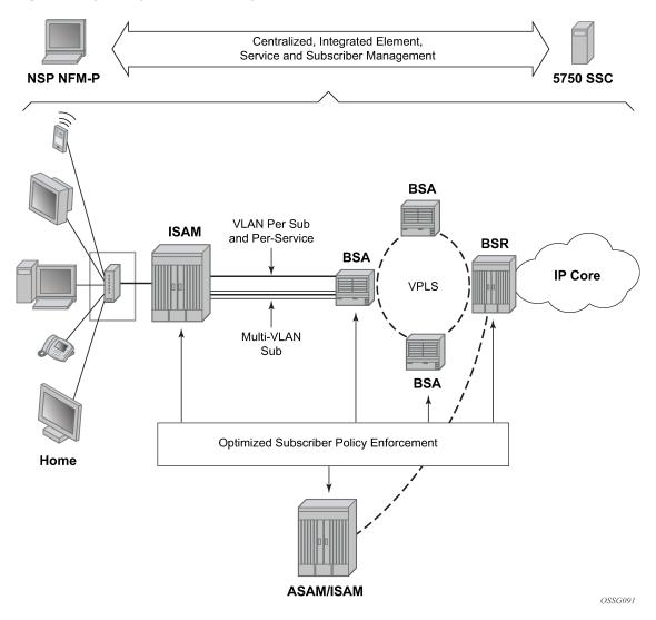
Figure 1: Triple Play Service Delivery Architecture
