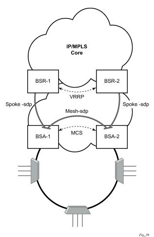
Typically, BTV service distribution is implemented in a separate VPLS service with a separate SAP per access-node. This extra VPLS is not explicitly indicated in Figure 104: Layer 2 CO dual homing - network diagram (and subsequent figures) but the descriptions refer to its presence.
