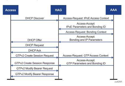
Figure 154: Bonding authentication
