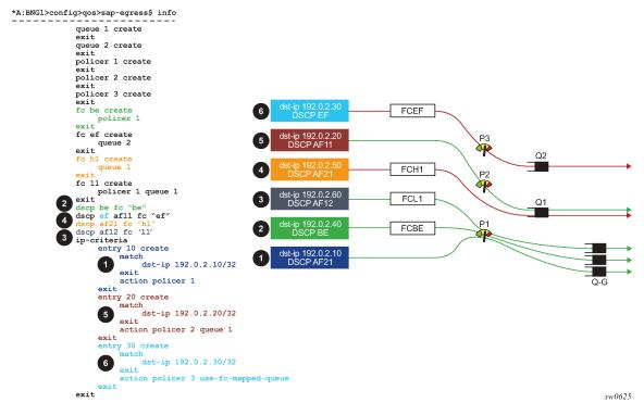
Figure 237: Egress statistics in relation to QoS deployment models
