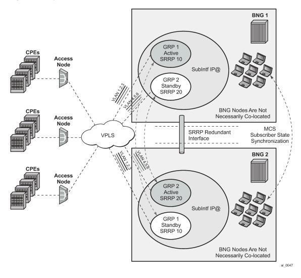
Figure 93: Fully redundant "stateful 1:1" model
