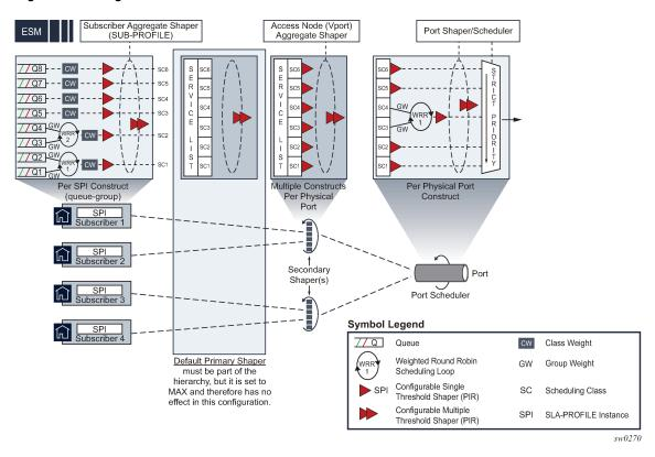
Figure 162: Single SPI mode
