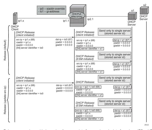
Figure 20: DHCP server IP address hiding, release
