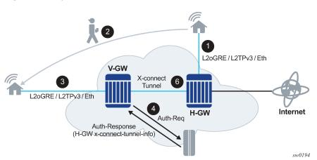
Figure 178: Dynamic tunnel x-connect for seamless inter-WLAN-GW mobility
