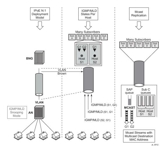
Figure 58: N:1 model - AN in IGMP snooping mode
