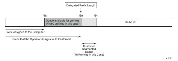
For example, a DHCPv6 server prefix pool contains an aggregated (configured) IPv6 prefix from which the delegated prefixes are carved out. In Figure 72: IPv6 prefix this aggregated IPv6 prefix has length of /48. In addition, the DHCPv6 server needs to know the length of the delegated prefix (in the above case /60). These two values are marking the boundary within which a unique delegated prefix is selected.
