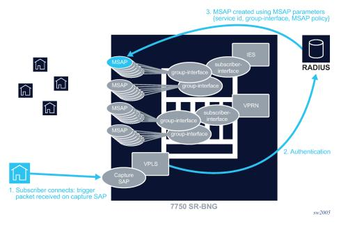
Figure 126: Managed SAP example configuration
