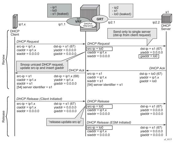
Figure 16: Relay unicast messages
