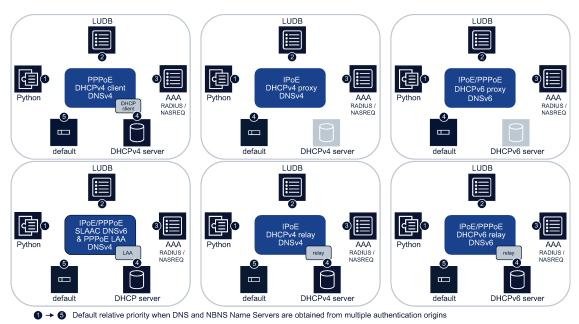
Figure 123: DNS and NBNS name server authentication origins
