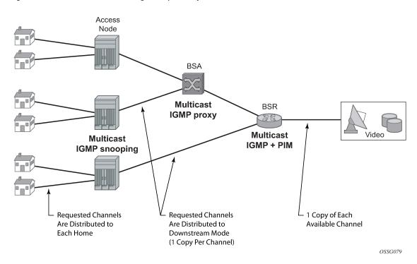
Figure 5: Distributed multicasting in Triple Play
