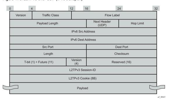
Figure 176: L2TPv3 over UDP (IPv6 transport)
