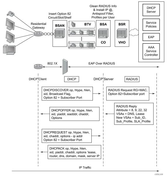
Figure 30: Aggregation network with DHCP to RADIUS authentication
