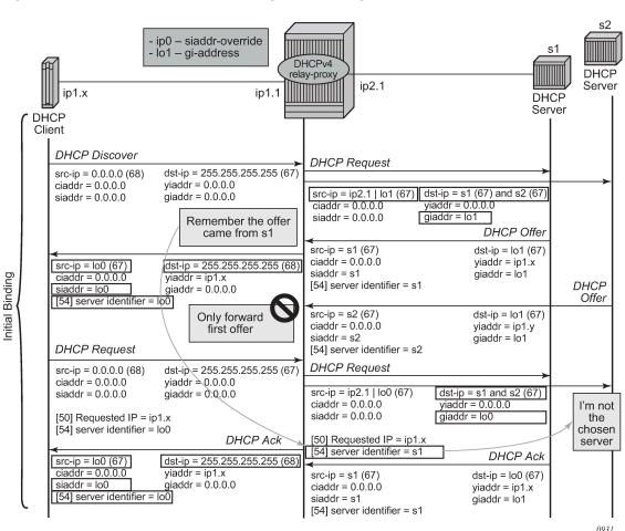
Figure 17: DHCP server IP address hiding/initial binding
