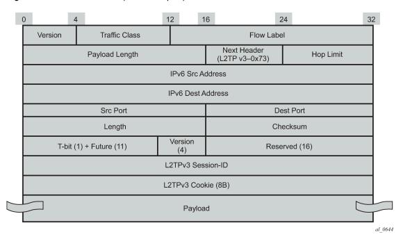
Figure 177: L2TPv3 over IP (IPv6 transport)
