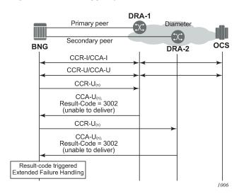
Figure 204: EFH trigger: protocol error
