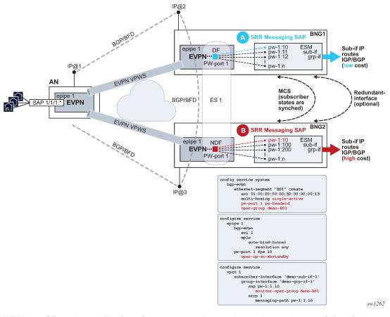
Figure 133: BNG multi-chassis redundancy with EVPN VPWS
