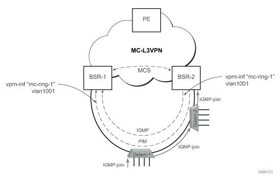
Figure 108: MC services in a Layer 3-Ring topology (a)
