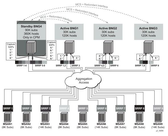
Figure 159: OMCR scenario with an aggregation network
