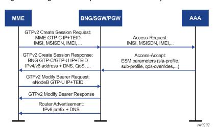
Figure 181: High-level example of GTP access setup
