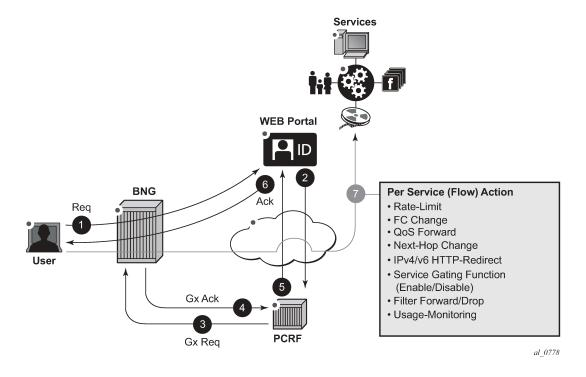
Figure 218: Generic use case for IP criterion-based policy change via Gx
