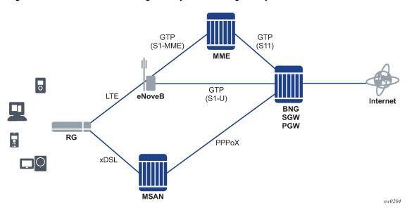
Figure 152: SGW/PGW/BNG integrated hybrid access gateway
