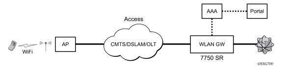
Figure 165: WLAN-GW functions on existing BNG
