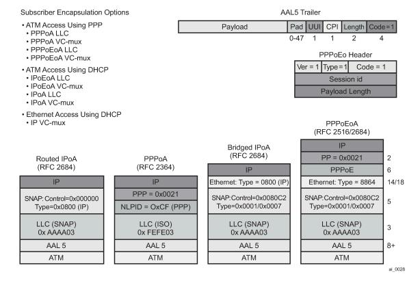
Figure 90: Access-loop-encapsulation sub-TLV
