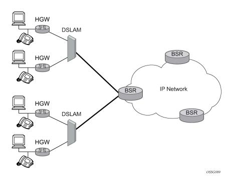
Figure 98: Aggregation network with direct DSLAM-BSR connection
