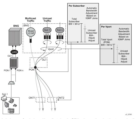
Figure 63: HQoS adjustment per subscriber and Vport
