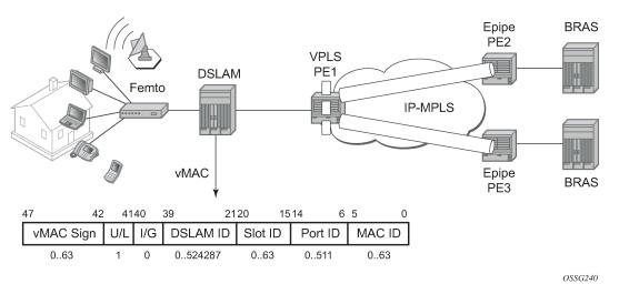
As the packet ingresses the DSLAM from the residential customer, the source MAC address (a customer MAC for one of its terminals or routers) is replaced by the DSLAM with a virtual MAC using the format depicted in Figure 7: VMAC subnetting topology.
