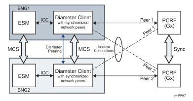
If the peering connections are colocated (Figure 234: Collocated peer connections), the preference parameter regains its meaning. In this case, Peer 1 is always selected over Peer 2.
