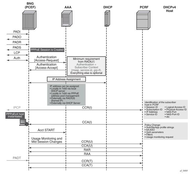
Figure 214: Message flow during PPPoEv4 host instantiation phase
