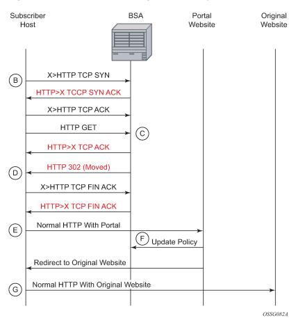
Figure 50: IP illustration of message flow in web portal redirect
