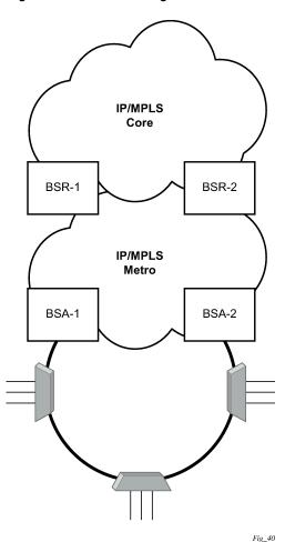
Figure 103: Dual homing to two PEs depicts dual homing to two different PE nodes. The actual architecture can be based on a single DSLAM having two connections to two different PEs (using MC-LAG) or ring of DSLAMs dual-connected to redundant pair of PEs.
