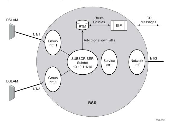
Figure 99: Detailed view of configurable objects related to Layer 3 subscriber interfaces
