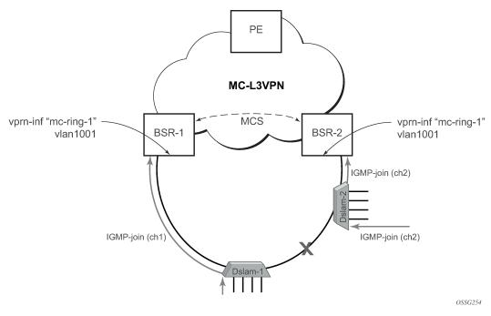
Figure 109: MC services on a Layer 3-ring topology (b)
