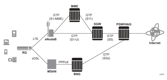
Figure 153: Sample hybrid access deployment
