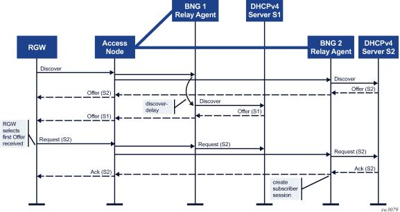
In Figure 28: DHCPv4 relay offer selection parameters, the DHCPv4 client on the RGW connects and broadcasts a DHCPv4 Discover message to obtain an IP configuration. Both the BNG 1 and BNG 2 relay
