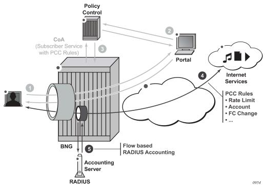
Figure 143: Example: PCC rule-based subscriber service
