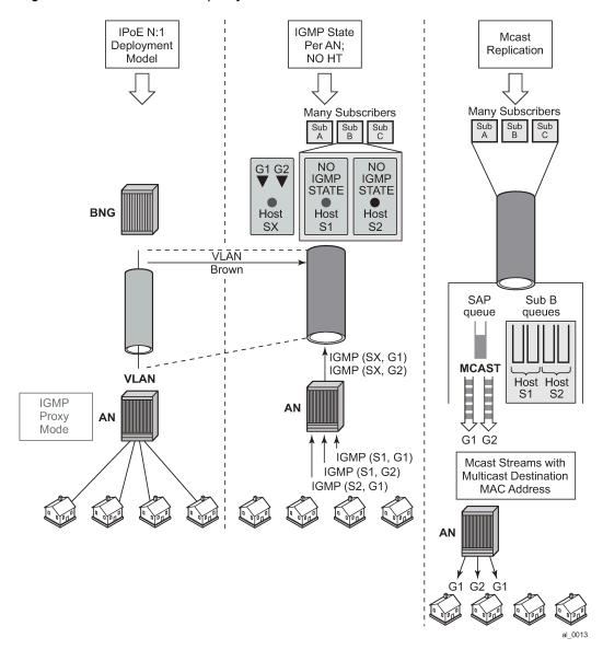
Figure 59: N:1 model - AN in proxy mode
