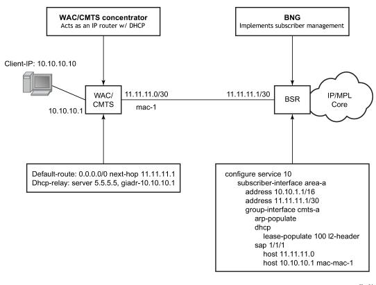
Figure 27: CMTS/WAC network configuration example
