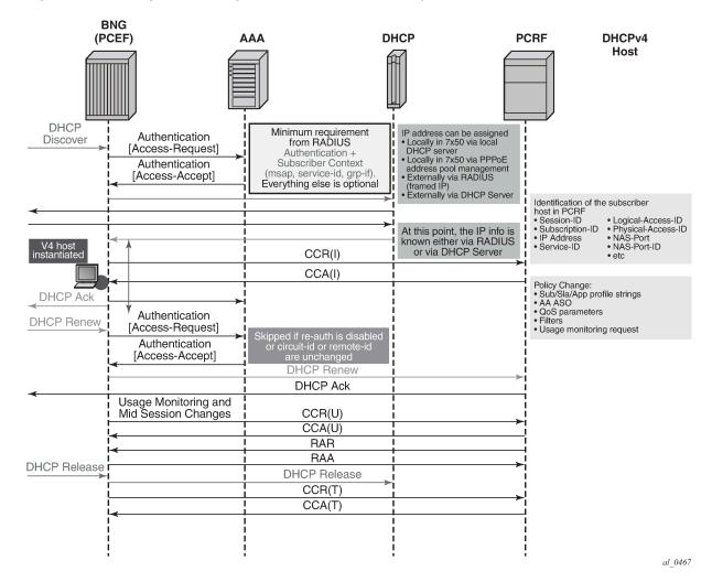
Figure 213: Message slow during DHCPv4 host instantiation phase
