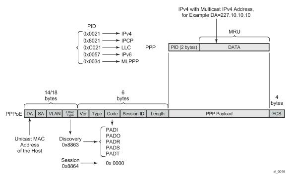
Figure 62: Multicast IPv4 address and unicast MAC address in PPPoE subscriber multicast
