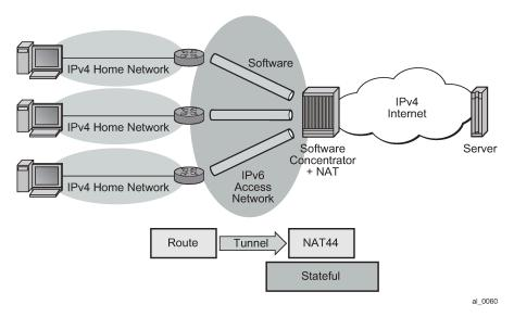
As shown in Figure 120: Dual-Stack Lite, DS-Lite has two components, a softwire initiator in the RG and a softwire concentrator, deployed in the service provider network, where control-less IP-in-IP (using protocol 4 - IPv4 in IPv6) is used for tunneling. When using control-less protocol, packets are sent on the wire for the remote softwire endpoint without prior setup of a tunnel.
