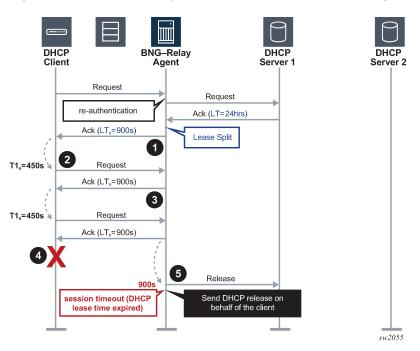
Figure 22: DHCPv4 lease split – DHCPv4 client disconnects ungracefully
