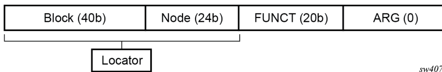
Figure 34: SRv6 SID encoding
