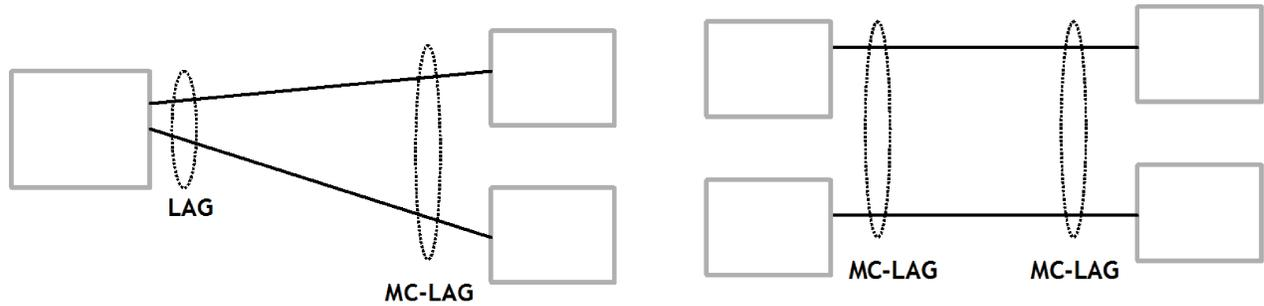
In case of a link failure, as shown in [Figure 34: LAG on access interconnection](#) and [Figure 35: LAG on access failure switchover](#), the switch over behavior ensures that all LAG-members connected to the same IOM as failing link become standby and LAG-members connected to other IOM become active. This way, QoS enforcement constraints are respected, while the maximum of available links is used.
