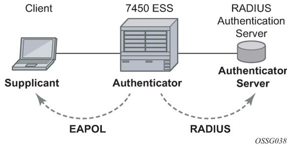
The authentication exchange is carried out between the supplicant and the authentication server, the authenticator acts only as a bridge. The communication between the supplicant and the authenticator is done through the Extended Authentication Protocol (EAP) over LANs (EAPOL). On the back end, the communication between the authenticator and the authentication server is done with the RADIUS protocol. The authenticator is therefore a RADIUS client, and the authentication server a RADIUS server.
