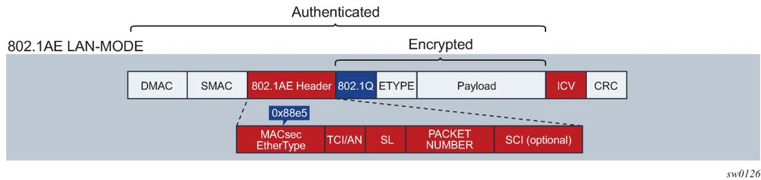
The forwarding on a MACsec packet is performed using the destination MAC address, which is in clear text.
