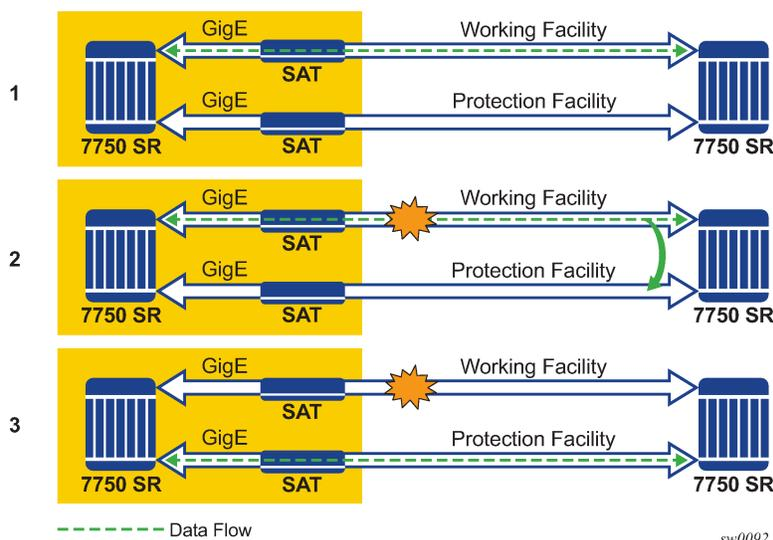
Note that “facility” in the router’s context refers to the physical line (including intermediate transport/switching equipment) and directly attached line terminating hardware (SFP module, MDA and IOM). “Circuit” is also a term used for a link/facility (working-circuit).
