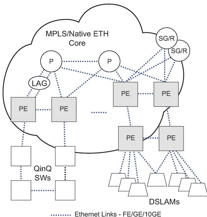
IEEE 802.1ab LLDP running on each Ethernet interfaces in between all the above network elements may be used to discover the topology information.
