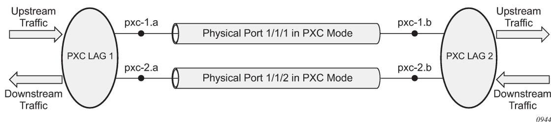
Although the configuration allows for a mix of port-based PXC and MAC-based PXC in a LAG, the configuration should be used in a production network only during a short migration period when transitioning from one type of PXC to the other. Outside of the migration, the PXC in a LAG should be of the same type, for example, a LAG should contain only port-based PXC or only MAC-based PXC but not both.
