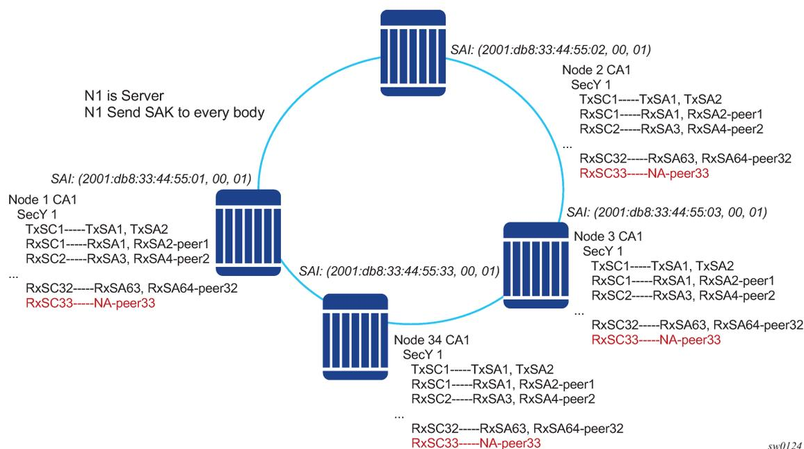
In Figure 11: Switch multi-point to switch multi-point topology, when the 34th node joins the multi-point topology, all other 33 nodes that are already part of this domain do not have any SAs to create an RxSC for this 34th node. However, the 34th node has a TxSC and accepts 32 peers. The 34th node starts to transmit and encrypt the PDUs based on its TxSC. However, because all other nodes do not have a SC for this SAI, they drop all Rx PDUs.
