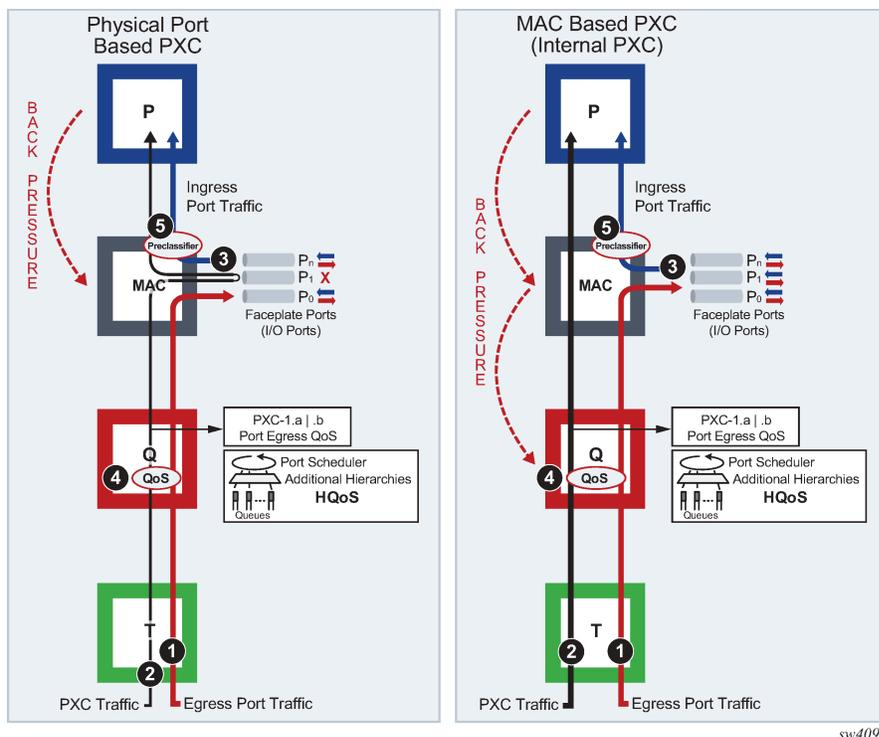
The physical port-based PXC configuration on the left side of [Figure 24: Interaction between PXC and non-PXC traffic](#), shows interaction of the three traffic streams on the forwarding complex with a PXC based on the faceplate ports. To manage congestion, the user-configured input can be exerted in points 4 and 5.
