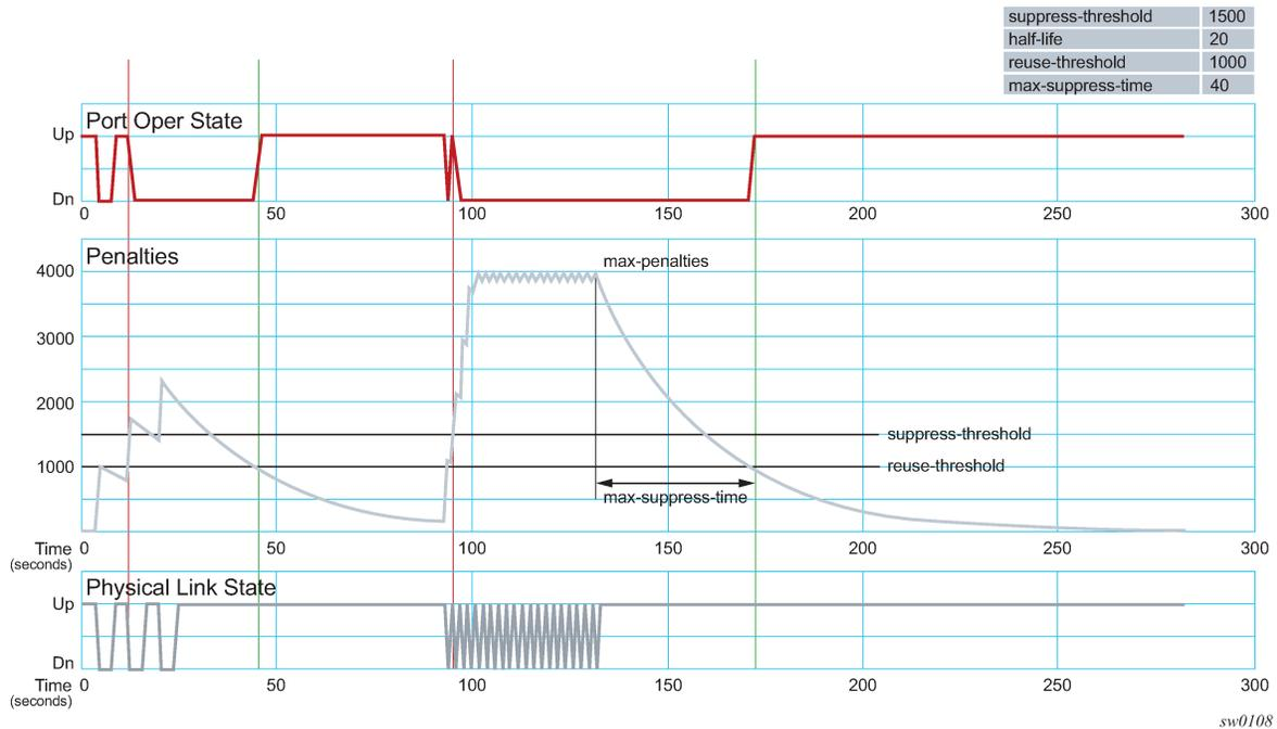
At time ( $t = 0$ ) in the preceding figure, the initial condition has the link up, the accumulated penalties are zero, the dampening state is idle, and the port operational state is up. The following series of events and actions occur.
