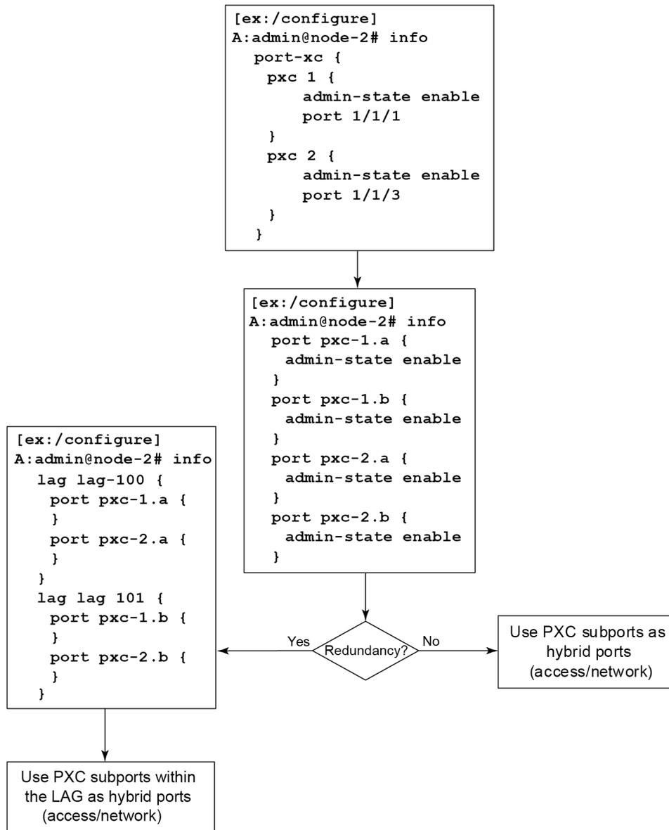
Figure 28: MD-CLI PXC configuration on internal loopback
