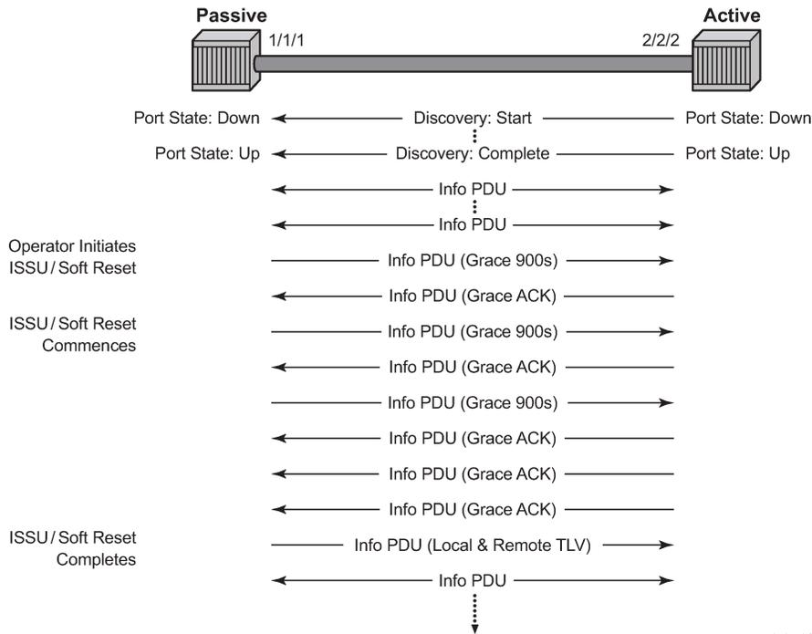
In [Figure 42: Grace TLV active node with soft reset](#), the Active node is experiencing the ISSU function on a node that supports soft reset capabilities.
