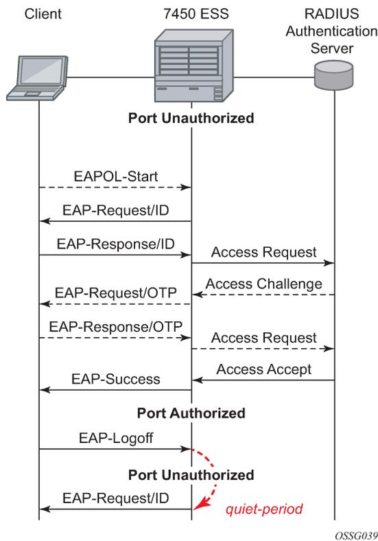
After receiving the EAP-Response/ID frame, the router encapsulates the identity information into a RADIUS AccessRequest packet, and sends it off to the configured RADIUS server.
