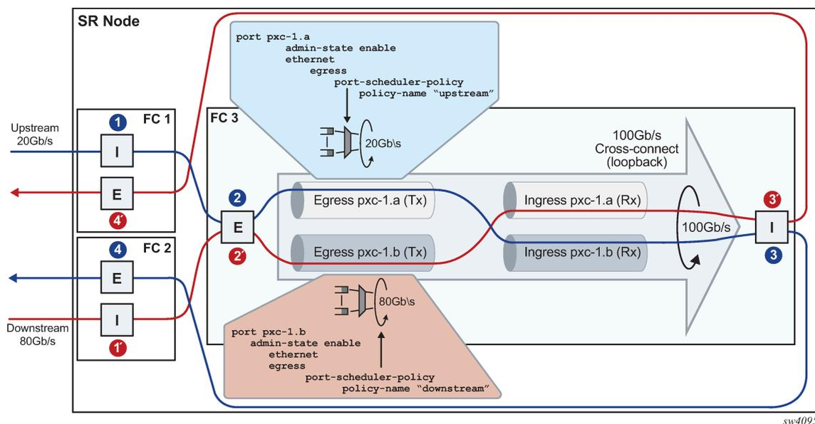
Traffic traversing PXC contains an overhead of 4 bytes per packet that are attributed to the internal VLAN tag used for PXC sub-port identification within the SR node. However, these 4 bytes are not accounted for in the configured QoS rates. Therefore, the operator should take this into consideration when configuring rates on QoS objects under PXC ports.
