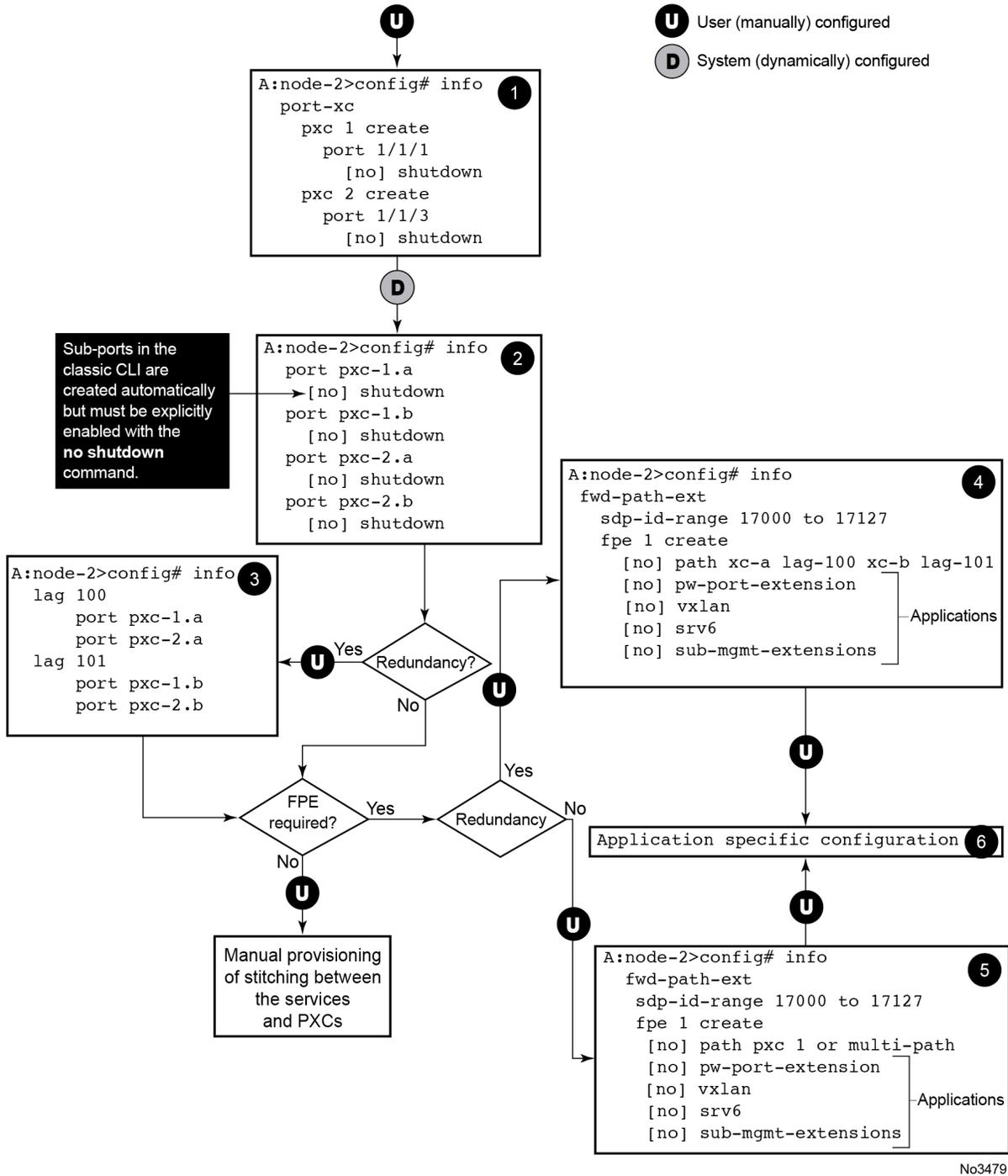
After the PXC sub-port or LAG is associated with an FPE object, the user cannot use CLI to create IP interfaces manually and SAPs under these PXC sub-ports or LAGs. Only the SR OS system is allowed to reference these PXC sub-ports or LAGs in internal IP interfaces and SAPs, as required by each application.
