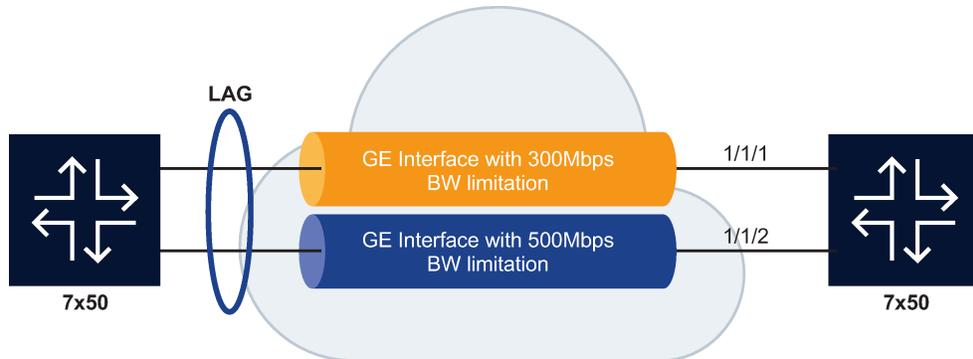
In this context, the user can configure the LAG using customized **hash-weight** values to adapt the flow distribution between LAG ports according to the bandwidth restrictions on each port. The following example shows the **hash-weight** configuration.
