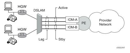
Figure 35: LAG on access failure switchover
