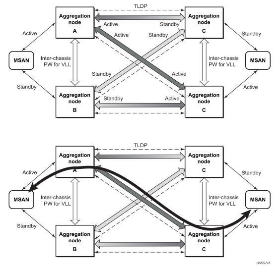
Figure 39: Point-to-Point (P2P) redundant connection through a Layer 2 VPN network
