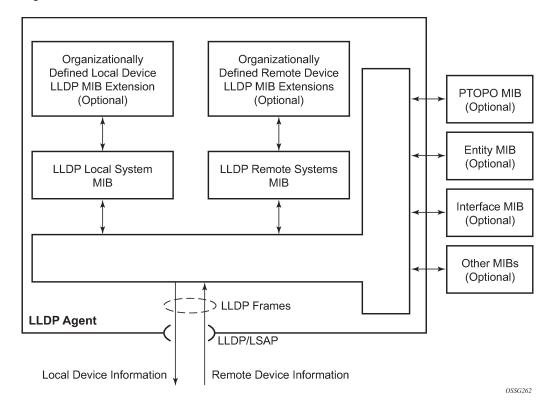
Figure 16: LLDP internal architecture for a network node
