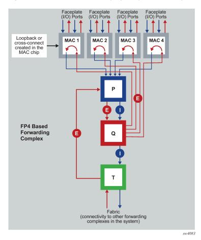
Figure 21: Internal cross-connect (loopback) in a MAC chip
