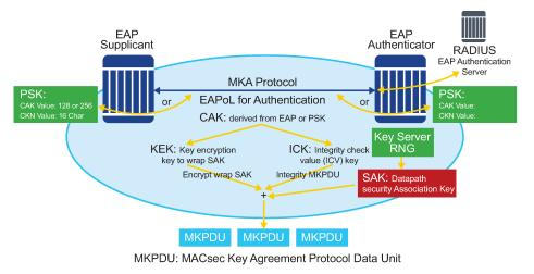
Figure 9: MACsec control plane and encryption
