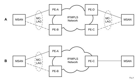
Figure 38: MC-LAG Layer 2 dual homing to local PE pairs
