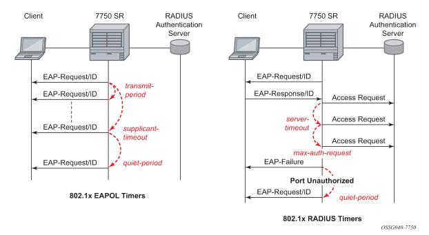
Figure 3: 802.1x EAPOL timers (left) and RADIUS timers (right)
