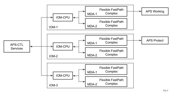
Figure 15: APS working and protection circuit example
