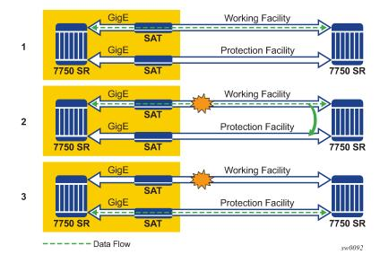
Figure 12: APS protection (single chassis APS) and switchover
