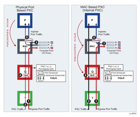
The physical port-based PXC configuration on the left side of Figure 24: Interaction between PXC and non-PXC traffic, shows interaction of the three traffic streams on the forwarding complex with a PXC based on the faceplate ports. To manage congestion, the user-configured input can be exserted in points 4 and 5.
