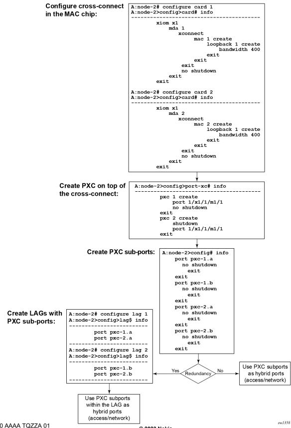
Figure 30: Classic CLI PXC configuration on internal loopback
