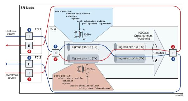
Figure 25: Bandwidth management on PXC sub-ports
