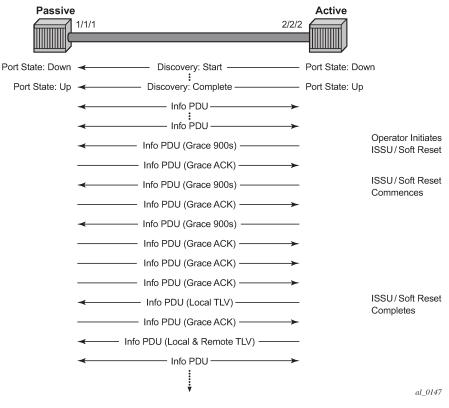
Figure 42: Grace TLV active node with soft reset
