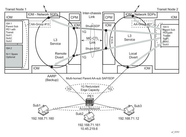
Figure 11: Multi-chassis asymmetry removal functional overview
