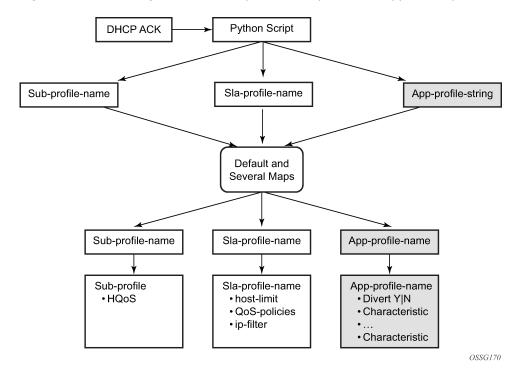
Figure 17: Determining the subscriber profile, SLA profile and application profile of a host
