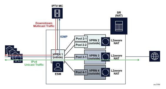
Figure 65: Downstream multicast traffic originated on the inside
