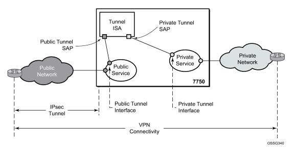
Figure 39: 7750 SR IPsec implementation architecture
