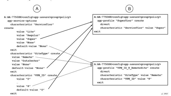
Then, the defined ASOs are used in the AQP definition to determine the needed treatment or policy (Figure 19: AQP definition example).
