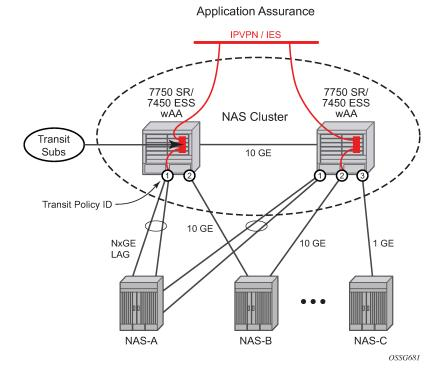
Figure 3: AA ISA inline identification, classification and control
