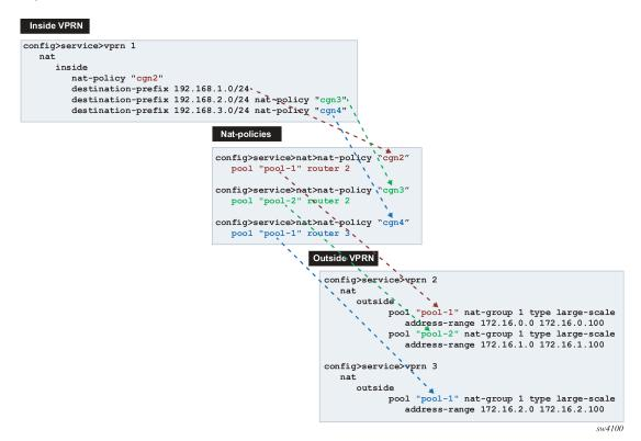
Figure 67: Logical representation of NAT routing through SR displays the logical configuration.
