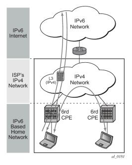
Figure 6: 6to4 in access network deployment
