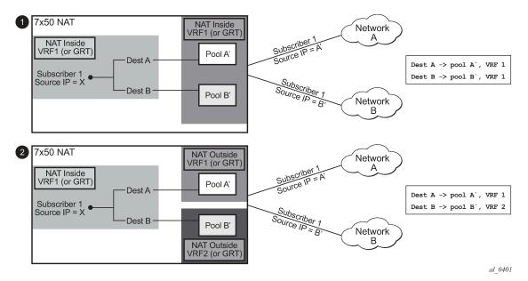
Diversion of the traffic to NAT based on the source of the traffic is shown in Figure 75: NAT pool selection based on the inside source IP address.
