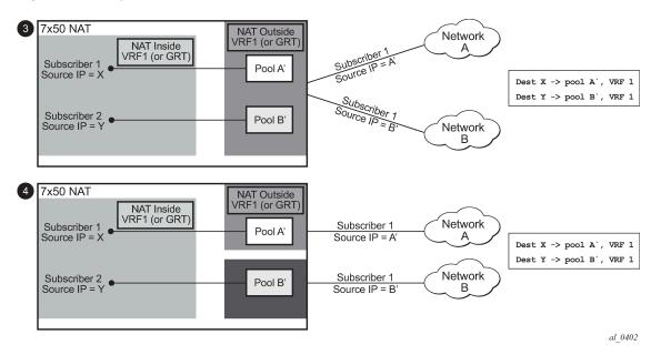
Figure 75: NAT pool selection based on the inside source IP address
