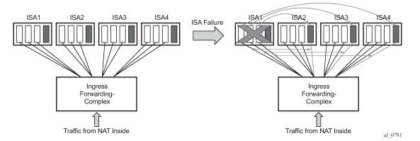
Figure 95: Load distribution in active-active intra-chassis redundancy model
