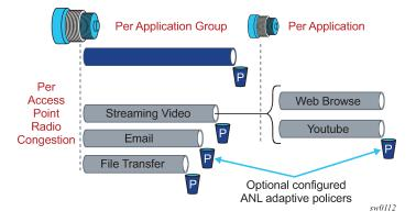
A DEM-GW is integrated directly into the WLGW using AA. The DEM-GW models the congestion points, called ANLs, that it learns from the WLGW subscriber attributes, and manages them accordingly to achieve the configured QoE/QoS target.
