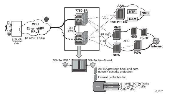
SAPs on the private side of Tunnel ISA are diverted to AA for firewall protection. If per eNB/ Femto Access Point (FAP) control is needed, then AA auto-configures/instantiate subscribers based on the "seen-ip" transit-AA subscriber model (no RADIUS interaction is required). This auto-creates a subscriber per eNB/ FAP. Alternatively, AA applies firewall rules to the diverted SAP (for all eNBs/FAPs) at the aggregate level (for all eNBs/FAPs).
