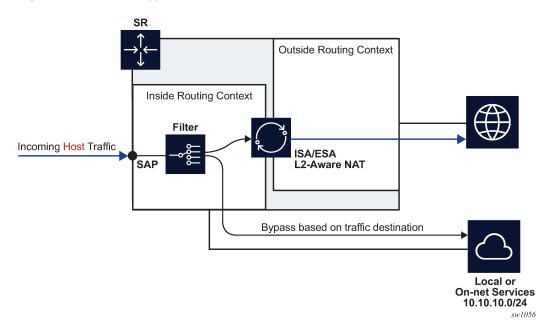
Figure 62: L2-Aware bypass based on traffic destination
