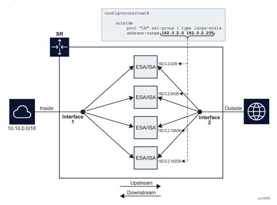
Figure 57: Load balancing over ISAs and ESAs
