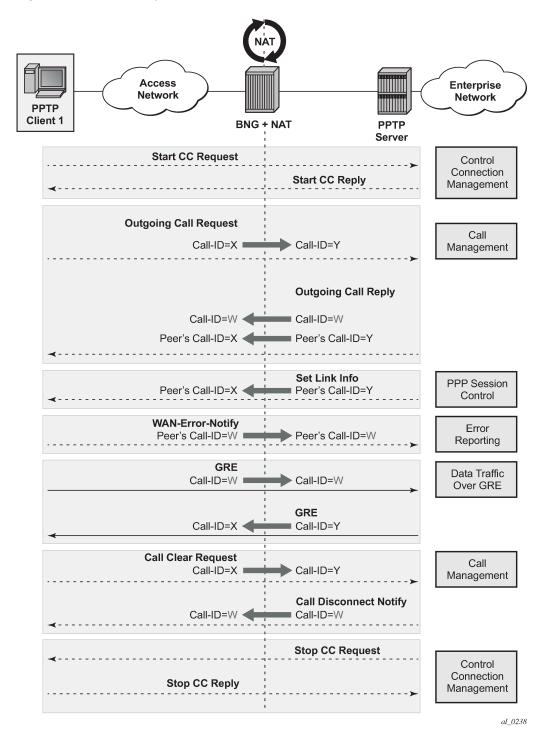
The scenario where multiple clients behind the NAT are terminated to the same PPTP server is shown in Figure 85: Merging of endpoints in NAT. In this case, it is possible that the source IP addresses of the two PPTP clients are mapped to the same outside address of the NAT. Because the endpoints of the GRE tunnel from the NAT to the PPTP server are the same for both PPTP clients (although their real source)
