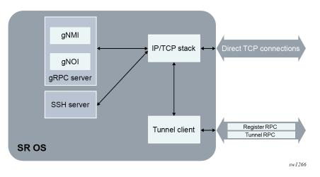
Figure 38: Internal SR OS architecture
