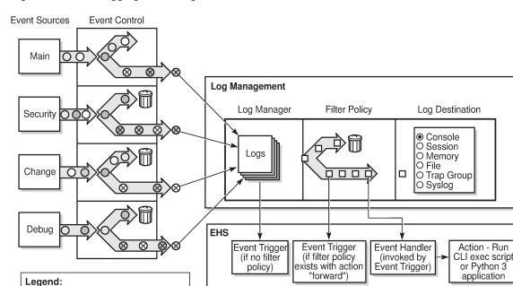
Figure 17: Event logging block diagram
