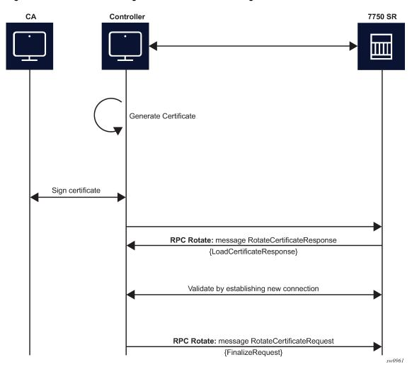
Figure 30: RPC Rotate message flow when CSRs are not generated on the SR OS node
