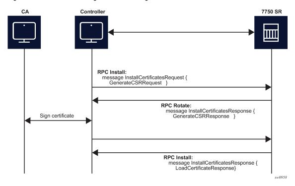
Figure 33: RPC install message flow for CSRs generated on the SR OS node
