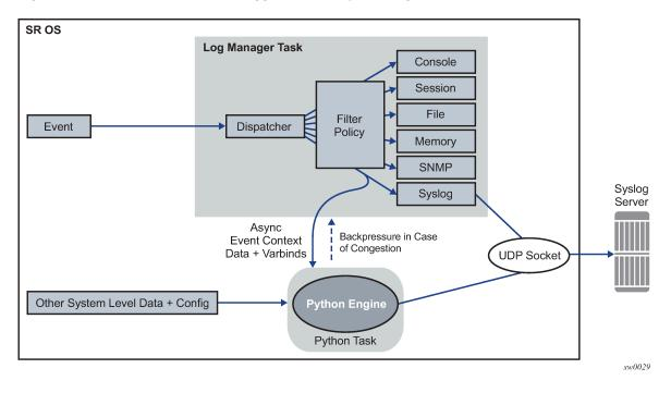
Figure 20: Interaction between the logger and the Python engine
