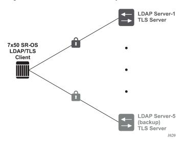
Figure 4: LDAP and TLS redundancy
