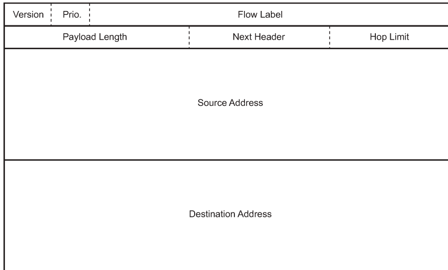
Figure 3: IPv6 header format
