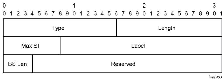
Figure 30: BIER MPLS Encapsulation sub-TLV format
