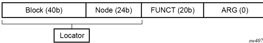
Figure 36: SRv6 SID encoding
