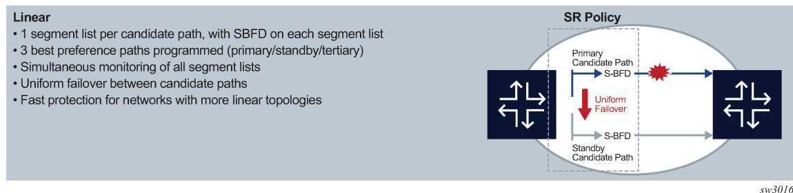
Figure 33: Linear protected SR policy with S-BFD
