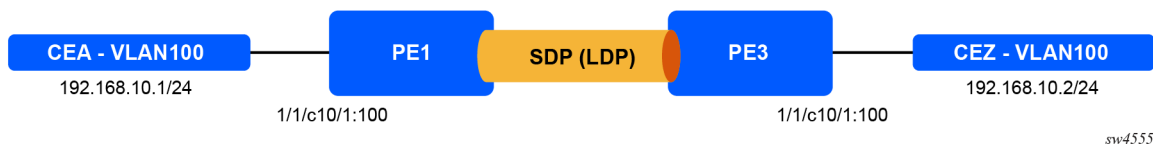
Figure 4: Epipe topology used in this example
