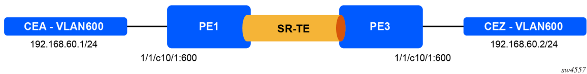
Figure 8: EVPN-VPWS topology used in this example
