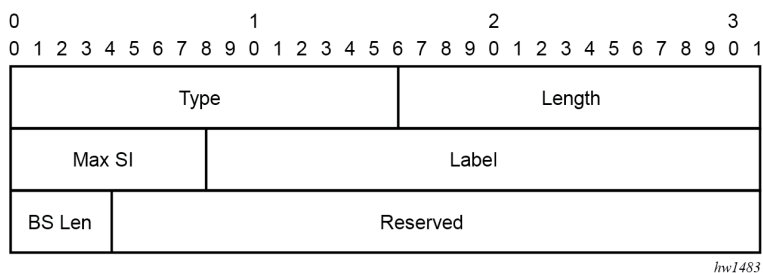
Figure 30: BIER MPLS Encapsulation sub-TLV format
