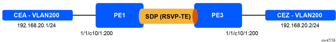
Figure 5: VPLS topology used this example
